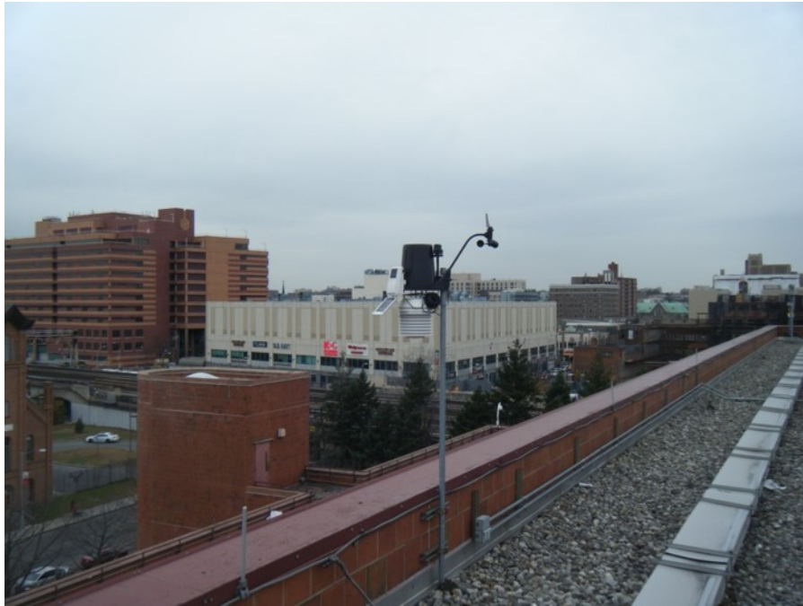
Figure 3: Roof-top Weather Station, with permanent power and network connections shown just to the right of the support pole.
