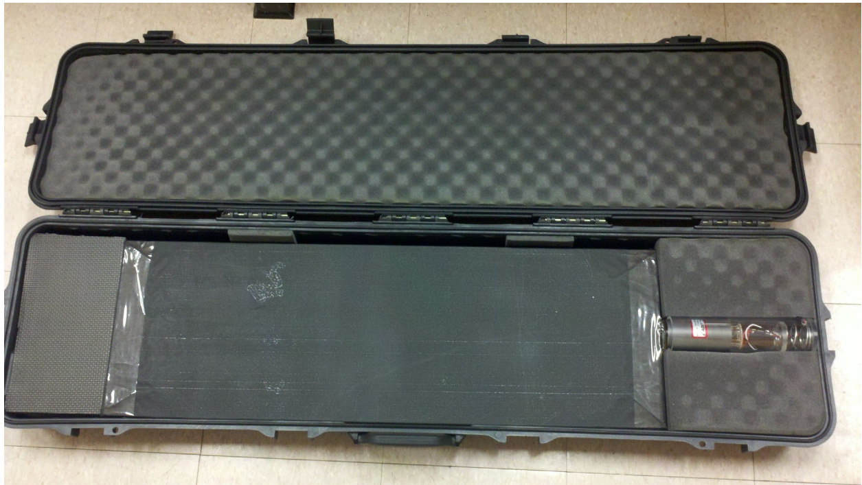
Figure 5: Scintillating paddle and PMT readout mounted in a firearms case.
