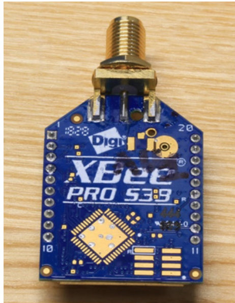
Fig. 2 The XBee radios serve as a wireless serial data connection allowing communication between the air and ground units
