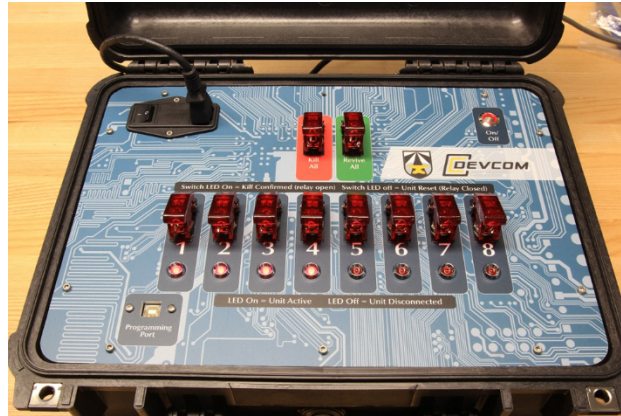
Fig. 9 The front plate contains the switches and LEDs that allow an operator to interface with the system and be updated on the system's state
