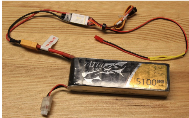
Fig. 6 The air units are powered independently of the UAS system by a battery and BEC so as to be a completely separate system
