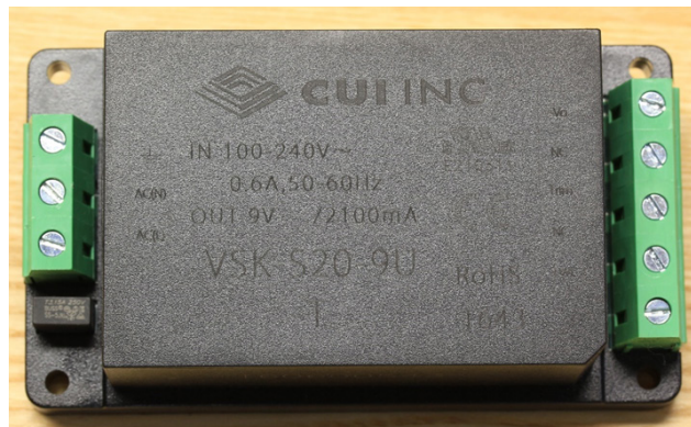
Fig. 12 The power supply converts standard 120-V AC power to DC power for the ground unit's systems
