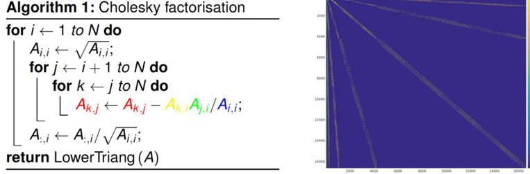
Figure 8: The algorithm. Skip entries of  $A$  (computational surrogate for  $\Theta$ ) outside of the sparsity pattern (i.e. skip all operations for which  $(k, j)$ ,  $(k, i)$  or  $(j, i)$  are outside of the sparsity pattern illustrated in the right figure).
