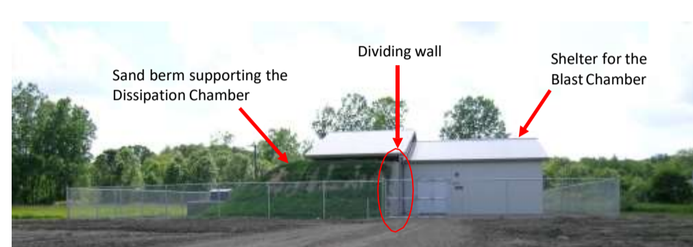
Figure 1. The ABC is a self-standing instrument composed by a blast chamber and a dissipation chamber. The blast chamber is sheltered by the structure on the right-hand-side, and the dissipation chamber is inside the sand berm on the left-hand-side.
