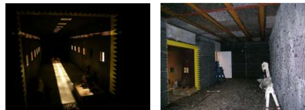
Figure 4. The end edges of the test section are serrated to start fragmenting the blast and to reduce noise (left) [4]. The blast is discharged into the dissipation chamber (right). The interior of this chamber is covered by 30 cm of rubber mulch to absorb and dissipate the energy of the blast.
