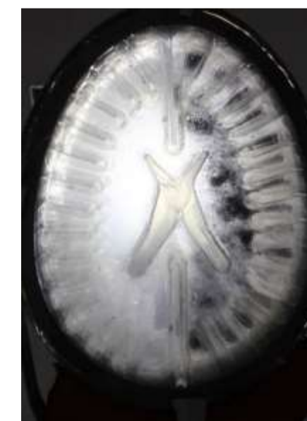
Figure 7. The current test object (1 st generation) is a simplified dual-material phantom based on the dominant geometrical features of an axial cut of a real patient. The materials are two different grades of polyacrylamide, tailored to approximate the mechanical properties of white and gray matter.
