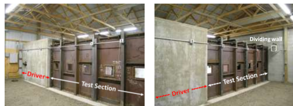
Figure 2. The Blast Chamber is composed by a Driver Section (1.5m deep steel cavity encased in reinforced concrete) and a steel-made Test Section with cross-section 2m x 2m and length 5.5m. Total length: 7m. The chamber protrudes through the dividing wall into the Dissipation Chamber.
