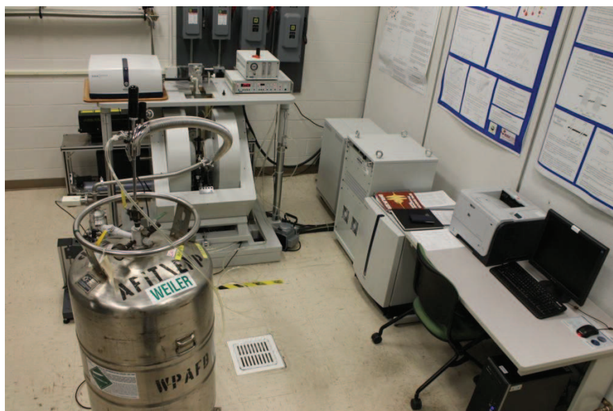
Figure 3.2. Experimental configuration of an EPR spectrometer for operation with liquid He.
