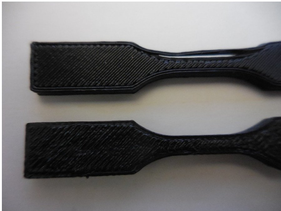
Fig. 11 Representative 3-D-printed specimen showing excess polymer along the gage section (this specimen was not used for testing)
