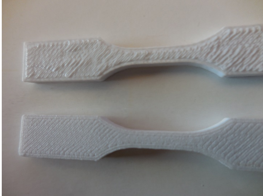
Fig. 10 Representative 3-D-printed specimen showing “rough” vs. “smooth” surface. This is a PLA tensile specimen.
