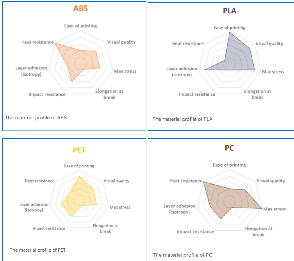
Fig. 4 Spider plots of the properties of common 3-D-printing polymers (image used with approval from https://www.3dhubs.com/knowledge-base/fdm-3d-printing-materials-compared 8 )
