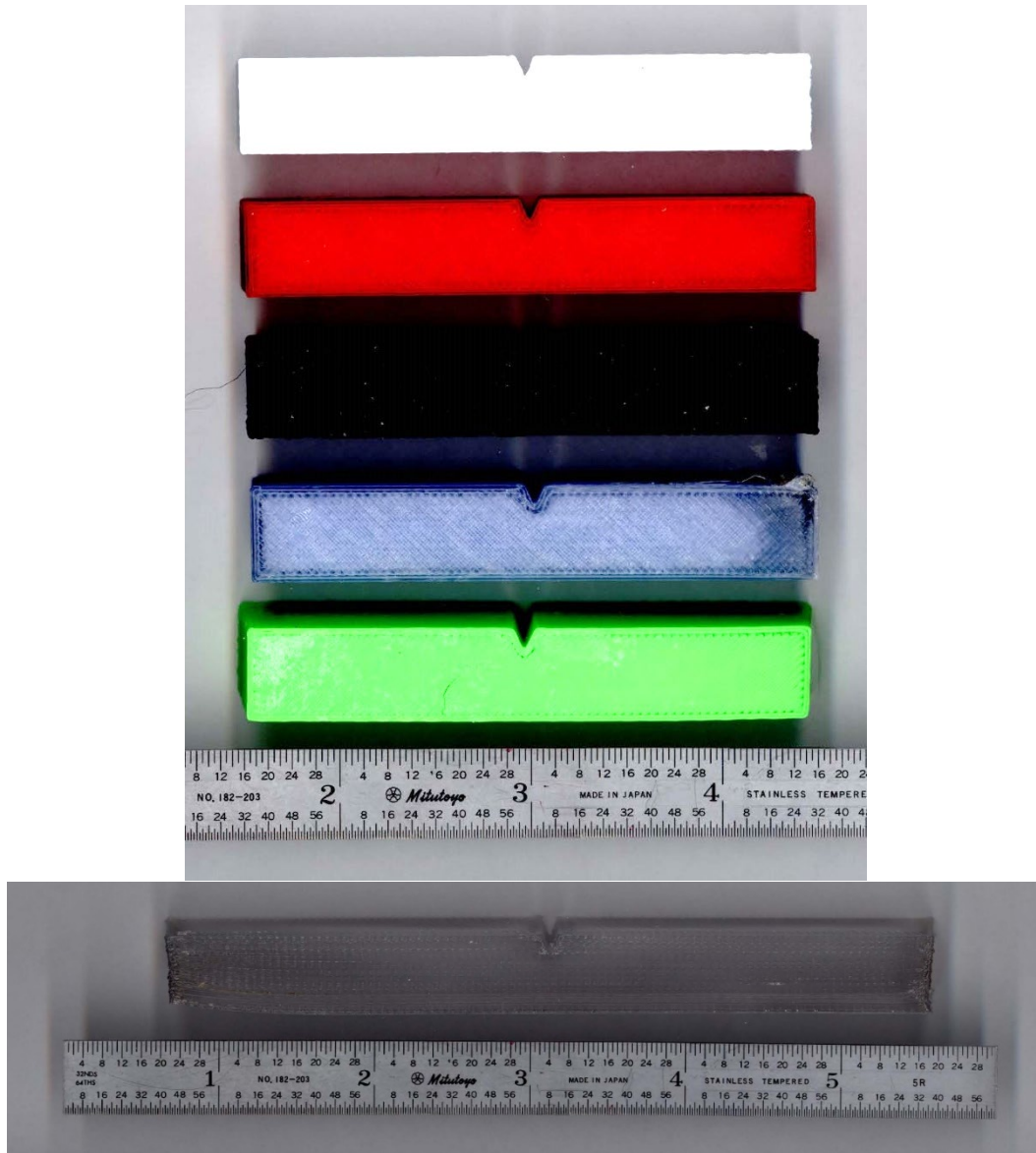
Fig. 8 Representative 3-D-printed impact specimens printed in PLA, PET-G, rABS, rPET, ABS (top to bottom in top photo), and PC (shown in bottom photo for better contrast)
