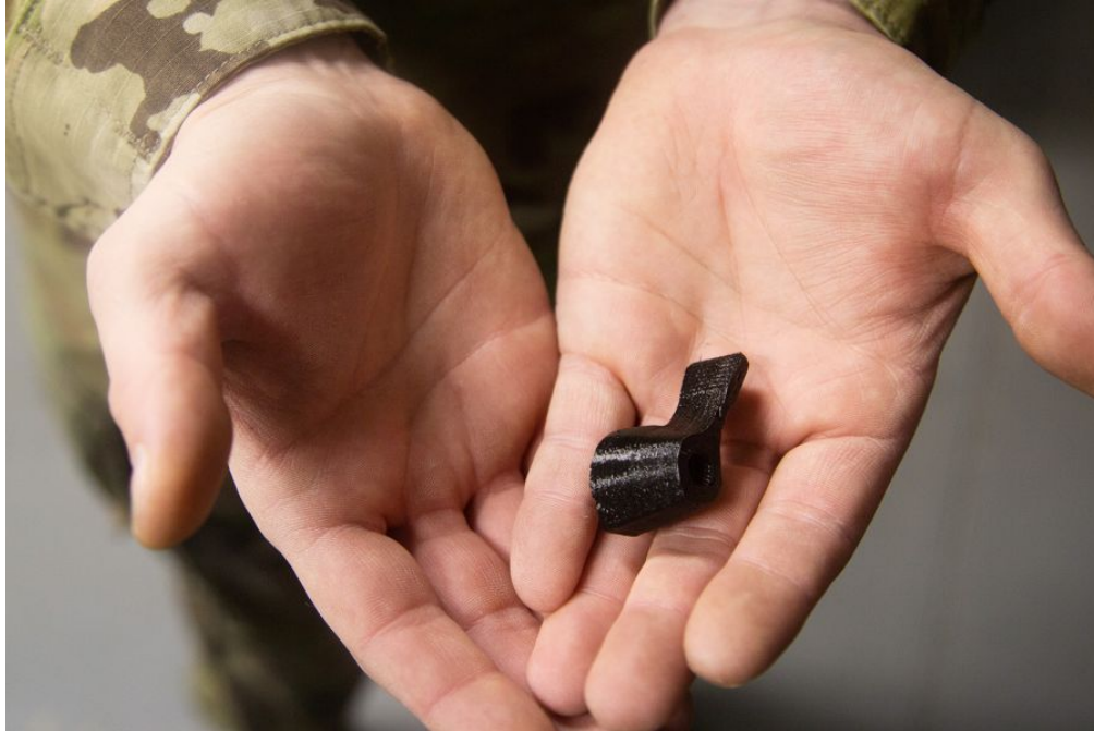
Fig. 2 A 3-D-printed Humvee ignition switch printed in the RFAB 5
