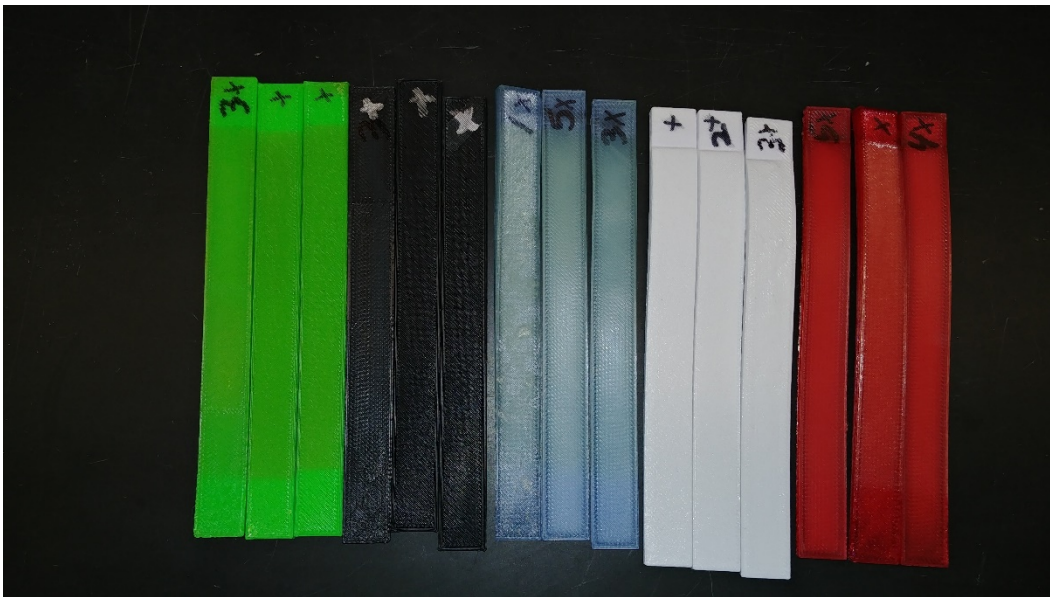
Fig. 16 Bending and discoloration of three-point bend specimens as a result of UV exposure. Samples deemed to have excessive bending were not tested.
