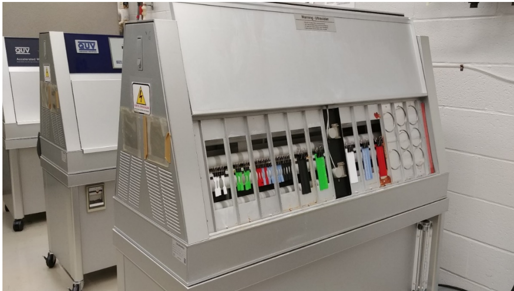
Fig. 14 Test setup used within the QUV equipment (tensile specimens on right; three-point bending specimens on left)
