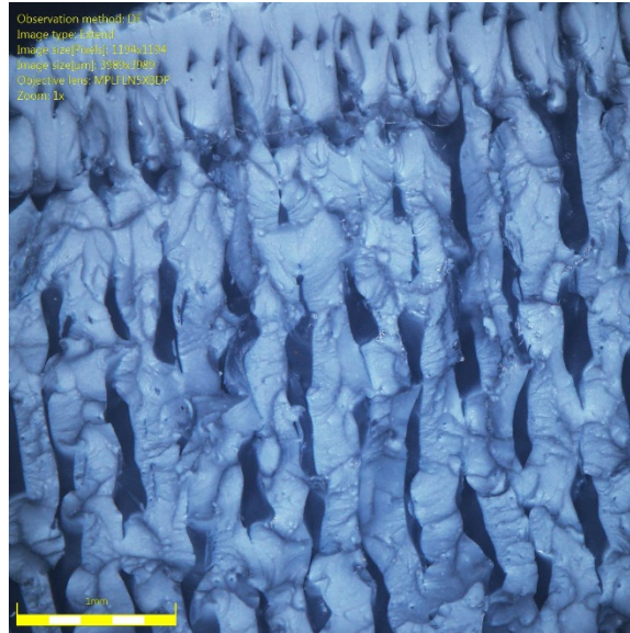
Fig. 49 Representative edge of rABS impact specimen fracture surface. Scale bar = 1 mm.
