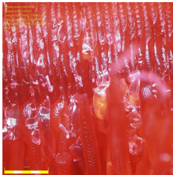
Fig. 50 Representative PET-G impact specimen fracture surface showing internal orange discoloring. Scale bar = 1 mm.
