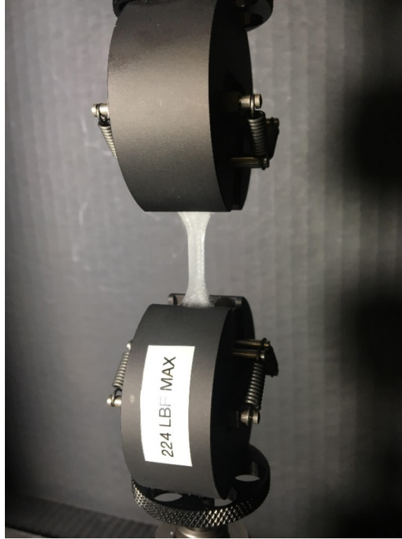
Fig. 23 A representative tensile specimen within the grips of the tensile test machine awaiting pull testing
