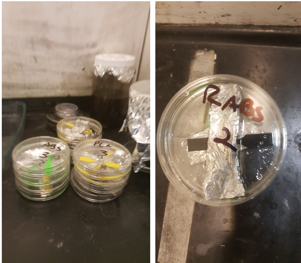
Fig. 17 Test setup for water immersion testing. Foil was needed to keep the specimens submerged.
