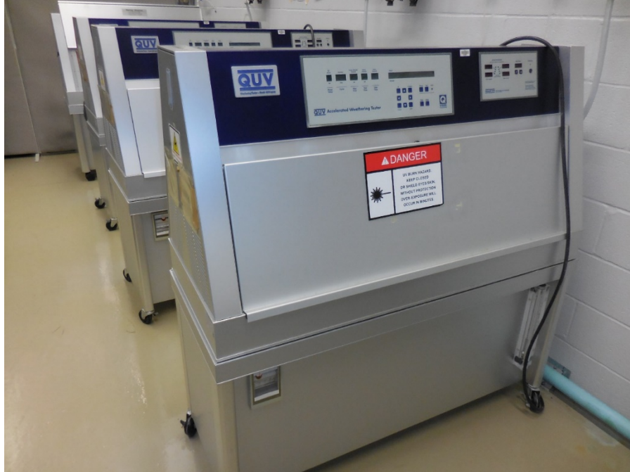
Fig. 13 QUV equipment used for UV exposure testing
