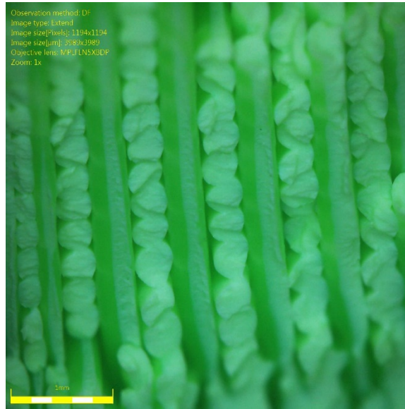
Fig. 47 Representative ABS impact specimen fracture surface. Structure represents the build pattern. Scale bar = 1 mm.
