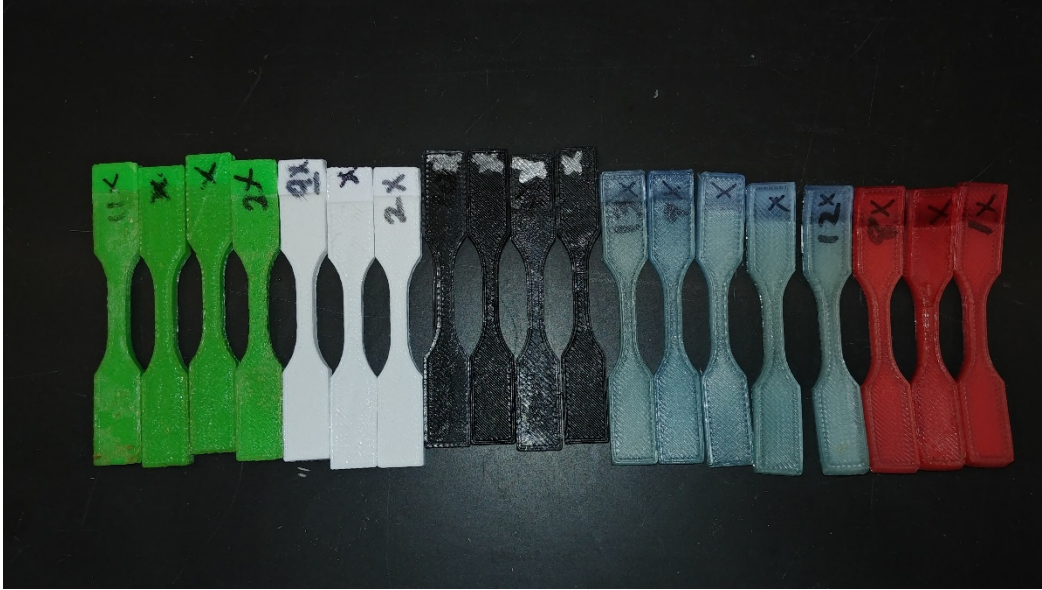
Fig. 15 Bending and discoloration of tensile specimens as a result of UV exposure
