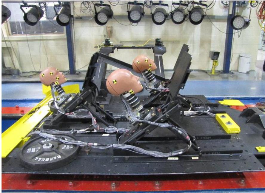
**Figure 6. ATD Head/Necks Mounted in -X-Axis Configuration: 40° Pitch, 0° Yaw**
