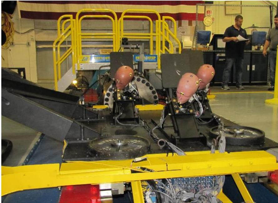
**Figure 4. ATD Head/Necks Mounted in +X-Axis Configuration: 40° Pitch, 45° Yaw**
