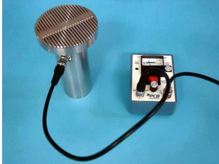
Figure 2. PCB Piezotronics microphone and power supply, per NASA's design.
