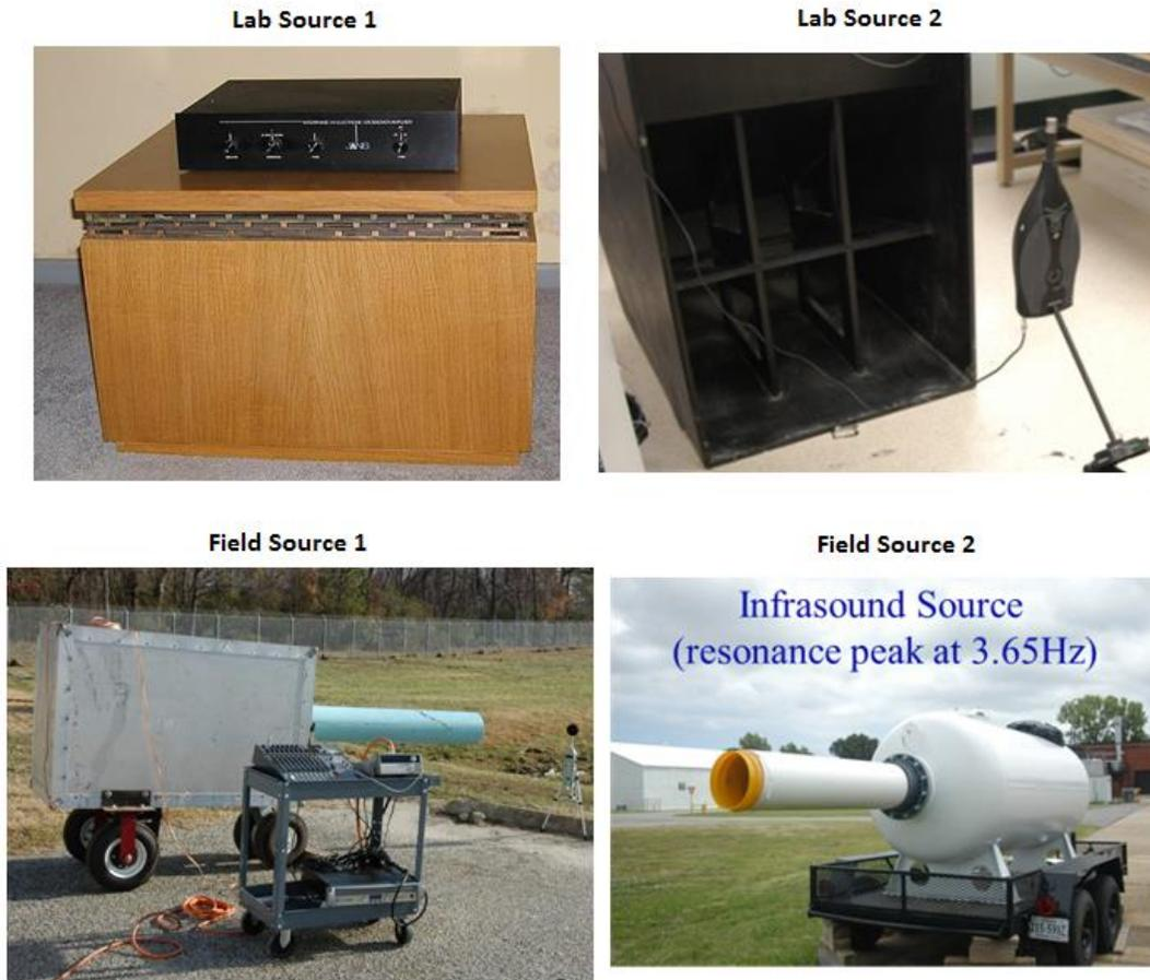
Figure 11. Infrasound sources used at NASA, Langley: 2 laboratory sources (top) and 2 outdoor field sources (bottom)
