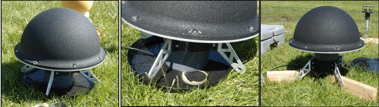
Figure 30. Different venting configurations evaluated in the field: Test 61 in tray of water (left), Test 62 in tray of water with air gap (center), and Test 63 spaced off ground on wood blocks (right).
