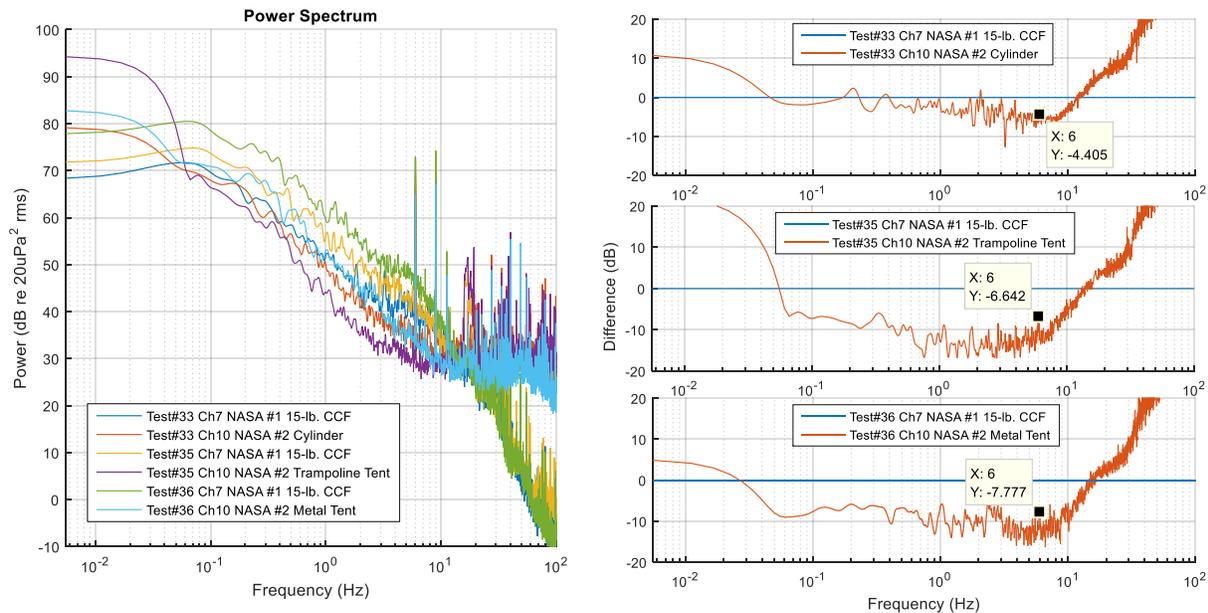
Figure 35. Comparison of NASA 15 lb. closed-cell foam windscreen to other windscreens
