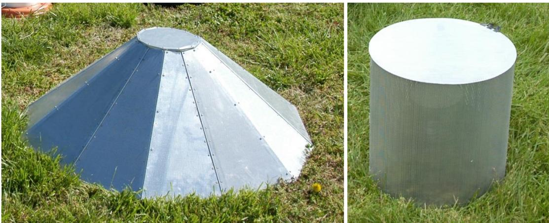
Figure 8. ARL perforated metal windscreens: tent style (left) and cylinder (right).
