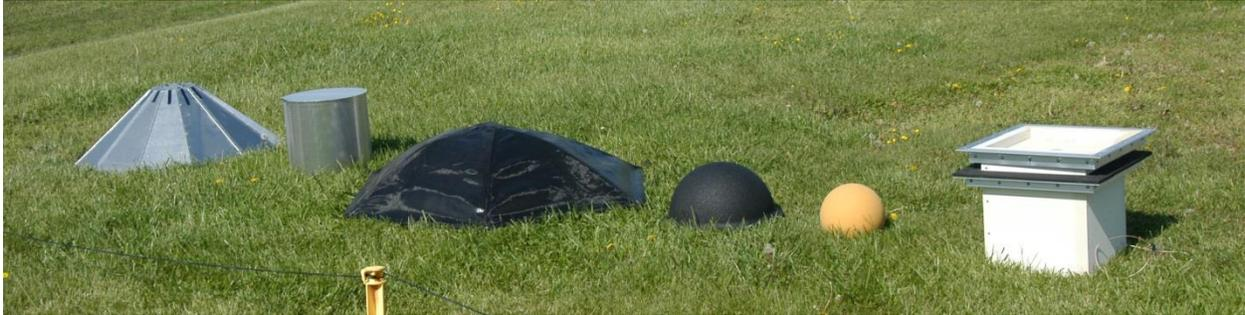
Figure 4. Comparison view of various windscreens used in testing. From left to right: ARL metal tent, ARL metal cylinder, Hyperion trampoline fabric tent, SSC Pacific CCF hemisphere, NASA CCF sphere, NASA CCF box.
