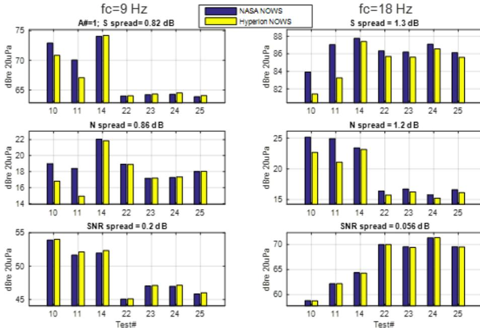
Figure 15. Comparison of NASA microphone and Hyperion microbarometer with no windscreens.
