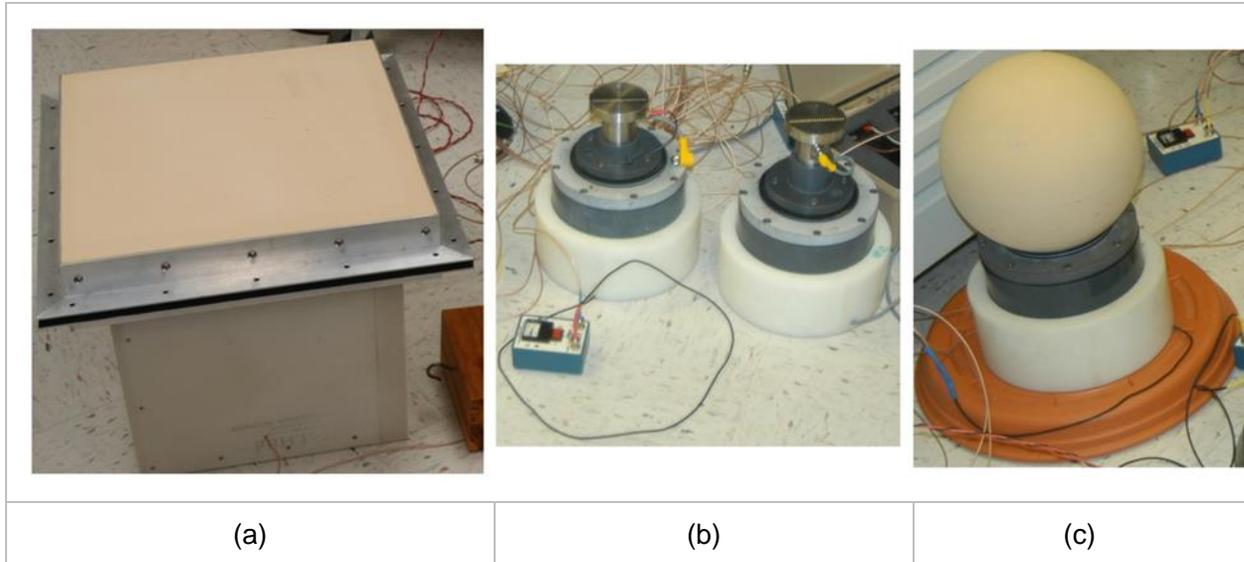
Figure 5. NASA CCF windscreens: box configuration (a), back chambers and microphones without windscreens (b), and complete back chamber with spherical windscreen (c)
