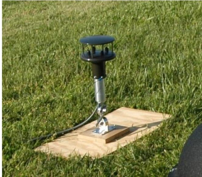
Figure 12. Gill ultrasonic anemometer and mounting base
