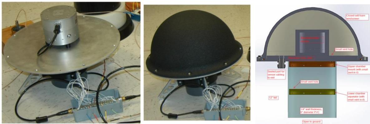
Figure 6. Hyperion microbarometer on base for hemisphere (left) and with hemisphere windscreen installed (center). Diagram of the windscreen assembly (right).
