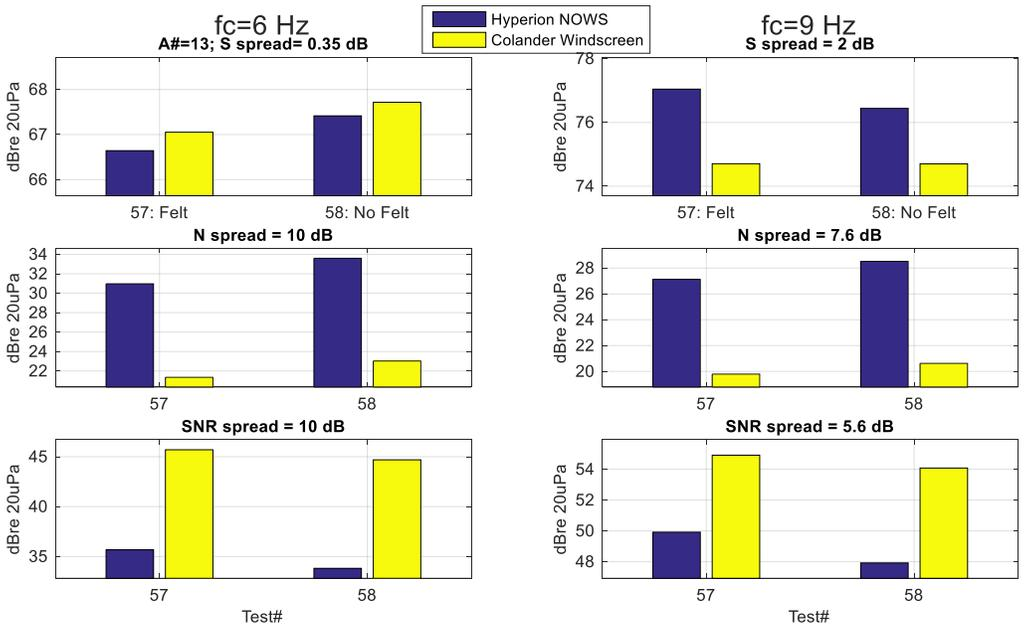
Figure 25. SNR comparison of Hyperion microbarometer with colander windscreen vs. NOWS.
