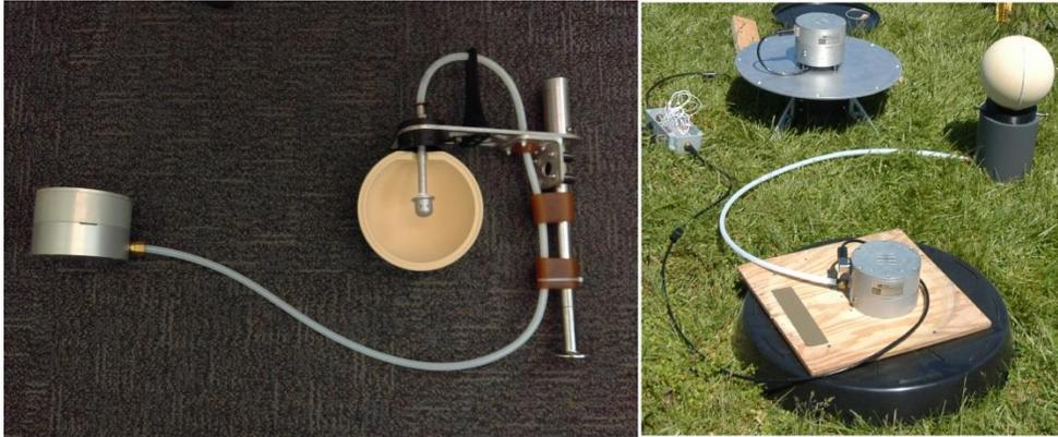
Figure 7. Hyperion microbarometer with remote acorn intake and closed-cell foam windscreen for USV installation (left) and with grounded back chamber as tested at NASA (right).
