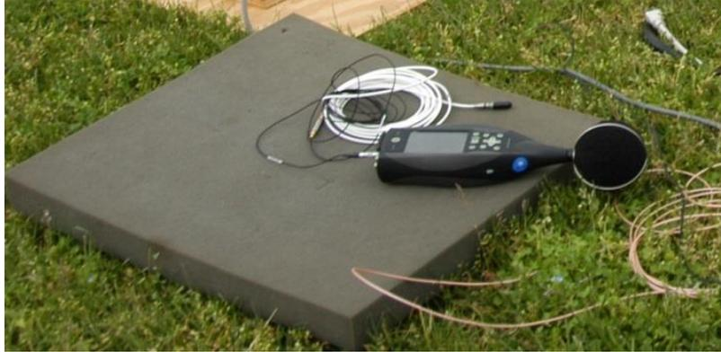
Figure 13. B&K 2270 with 4189 microphone with spherical open-cell foam windscreen and 8103 hydrophone.
