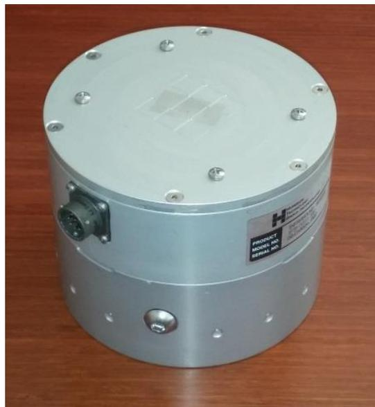
Figure 3. Hyperion IFS-5311 microbarometer.
