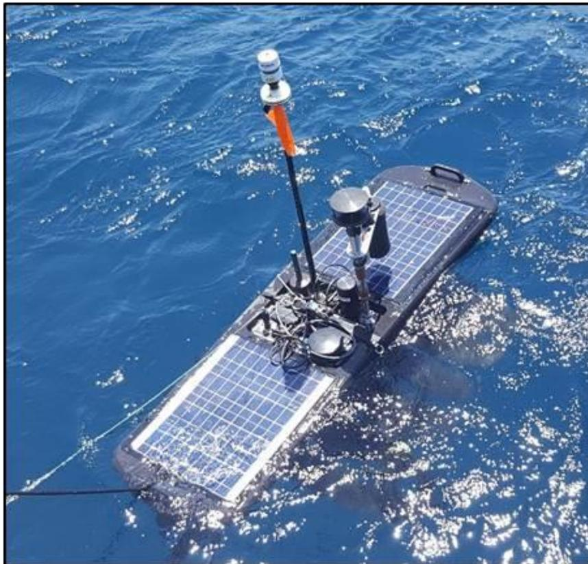
Figure 1. SV2 Waveglider with infrasond sensor package installed.
