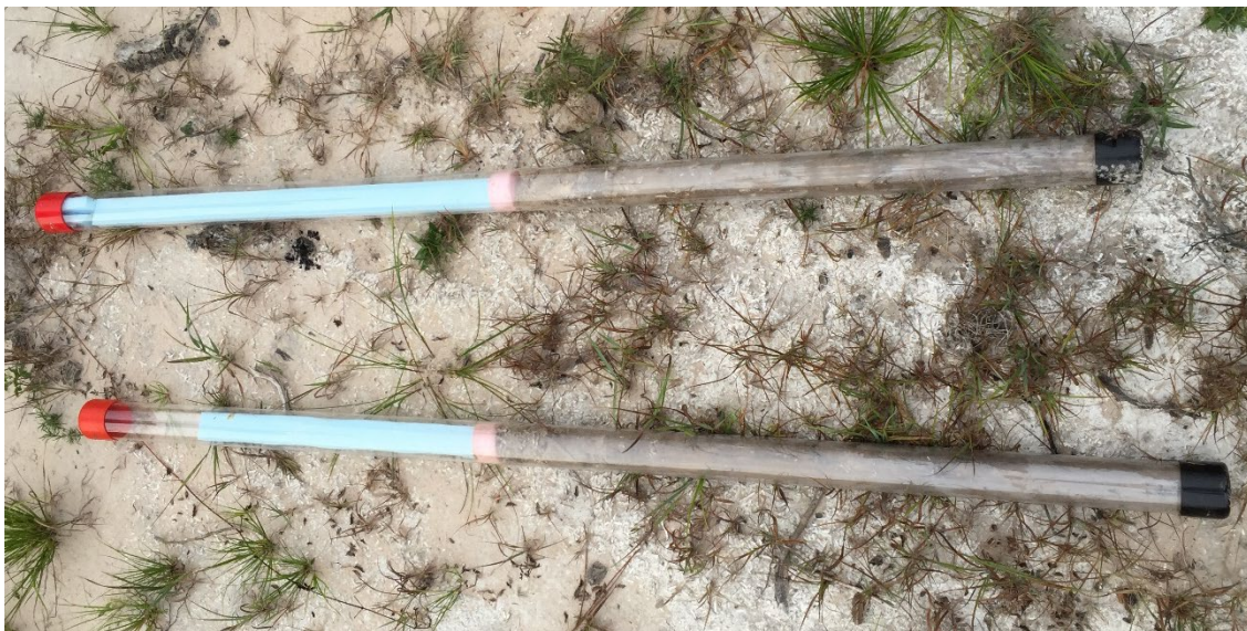
Figure 23. Soil cores stored in tubes to be sectioned by depth and analyzed.
