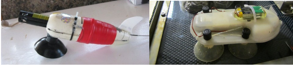
Figure 2-2. Two different suction-cup-attached tags used in the study. Left: The 3MPD3GT tag produced by Little Leonardo, Tokyo, Japan. Right: The Dtag produced by the Woods Hole Oceanographic Institution, USA. Both devices sense high-rate acceleration data which enables identification of glides, and pressure to measure animal depth during glides. The 3MPD3GT device has a flywheel speed sensor to measure speed changes during glides, while for the Dtag speed is measured using the change of depth divided by \sin(\text{pitch}) which works well for relatively vertical transit during descent and ascent phases of dives (Miller et al., 2004).
