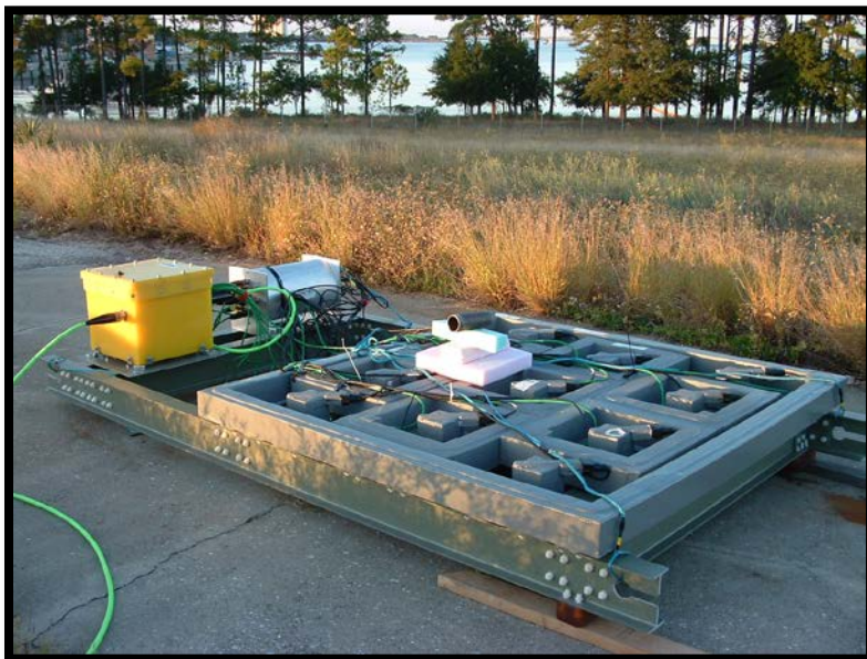
Figure 2. Photograph of Underwater Advanced Time-Domain Electromagnetic System
