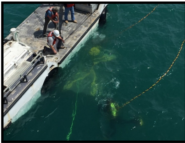
Figure 12. Surface Supplied Diver Operations from LARC, Including EM System Maneuvers and Test Item
