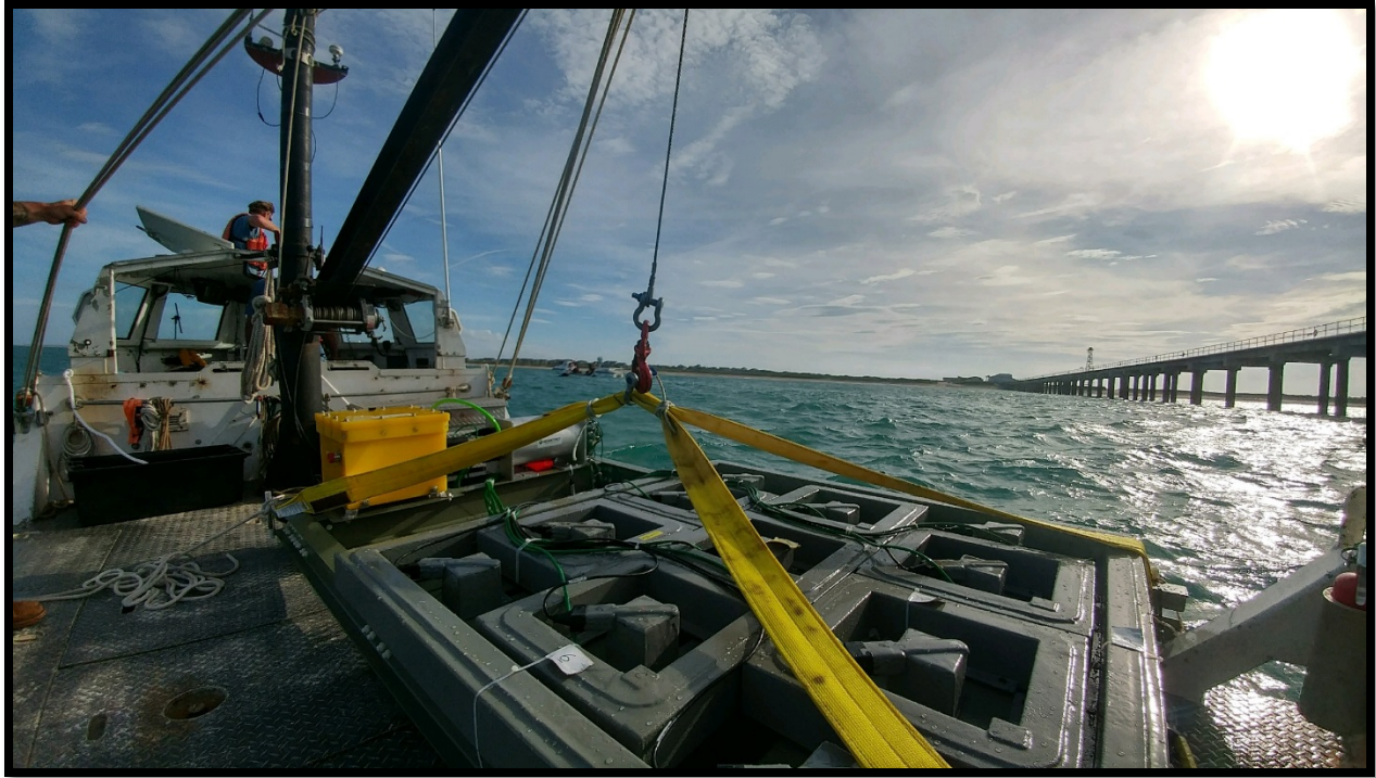
Figure 2. Photograph of the Underwater Advanced Time-Domain Electromagnetic System
