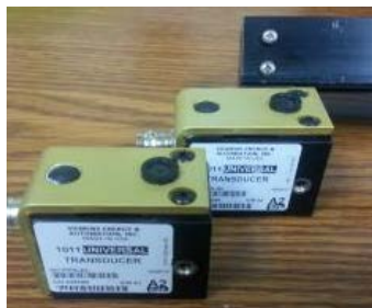
Figure 5.9. Temporary Installed Ultrasonic Meter and Its Accessories.
