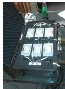
(d) Velocity probe transducer in custom built case
