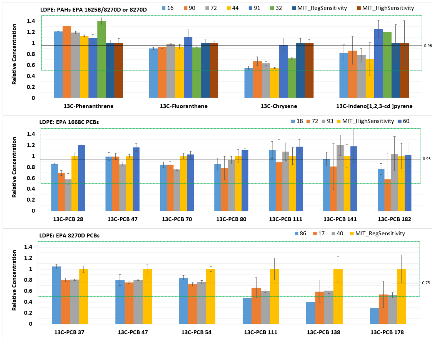
Figure 3. PRC Pre-loaded LDPE polymeric sampler results in relative units ( C_{reported}/C_{known} ). PCB congeners analyzed by high-sensitivity and regular-sensitivity methods are respectively shown in the middle and bottom; PAHs analyzed by regular- and high-sensitivity methods are shown at the top of the figure. The \pm 50\% of known concentration performance criteria is highlighted in green. Average results for each data set are shown as black lines with average values to right.
