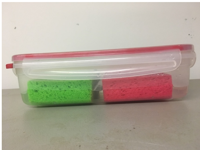
Figure 2-6. Moisture box for reference sample storage.
