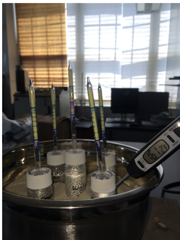
Figure 3-2. Preliminary colorimetric contaminant test.
