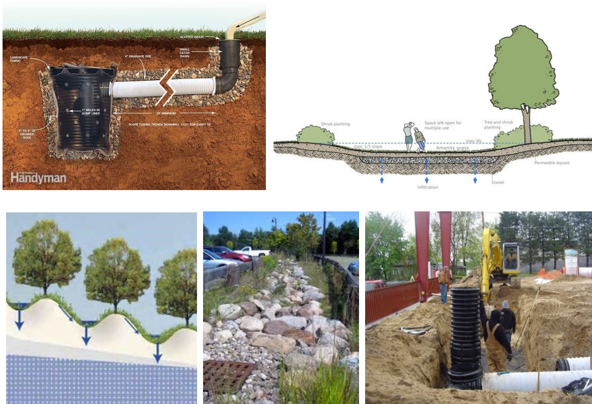
Figure 14. Clockwise from top left: diagram of a dry well, infiltration basin, subsurface infiltration bed, infiltration trench, and infiltration berms.
