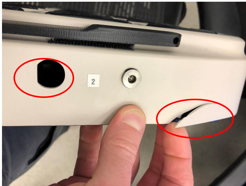
Figure 15. Damage in red circles to the charging dock USB connector and the plastic frame itself.
