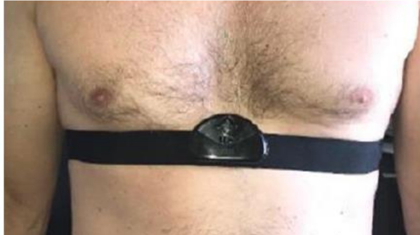
Figure 1. The Open Body Area Network – Physiological Status Monitoring (OBAN-PSM) system as worn on the body.
