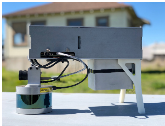
Figure 1. The Localization and Mapping Platform (LAMP) with a custom multi-planar CdZnTe (CZT) crystal array, MiniPRISM, which enables reconstructions that leverage Compton as well as coded-aperture imaging.
