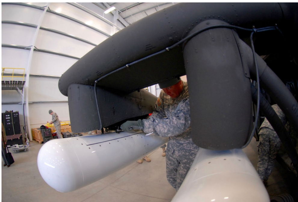
Figure 1. installation of ARDIMS (Aerial Radiation Detection Identification and Measurement System) on a UH- 60. ARDIMS consists of gamma and neutron detecting pods. During the National Technical Nuclear Forensics (NTNF) mission, it is used to map the fall-out field from a nuclear detonation and plan interagency missions for sample collection.
