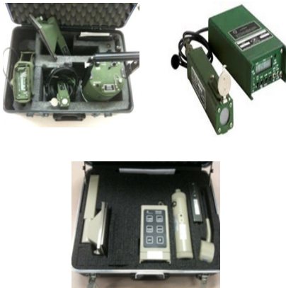
Figure 1. The RDS replaces the Army's AN/PDR-77 RADIAC and AN/VDR-2, the Air Force's ADM-300 Suite, and the Navy's AN/PDQ-1 Multifunction RADIAC (not shown). Images are reproduced with permission from Canberra.
