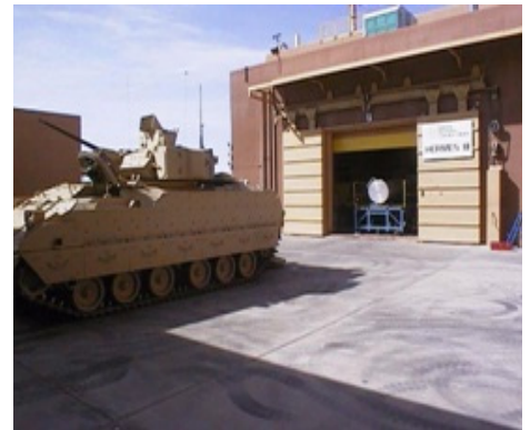
Figure 1. An example of a system level threat level simulator: Gamma dose rate system test of a M2 Bradley fighting vehicle at Sandia National Laboratories' HERMES III facility. See reference [2].
