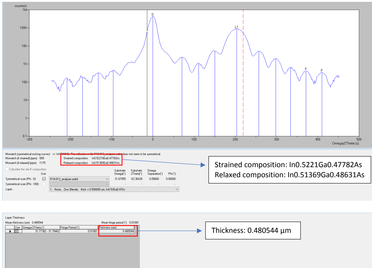
Figure 11: Calculation results on Epitaxy® for InGaAs grown on InP.
