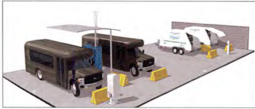
Figure 2.3.5: HAVO 350 Bar dispensing station.
