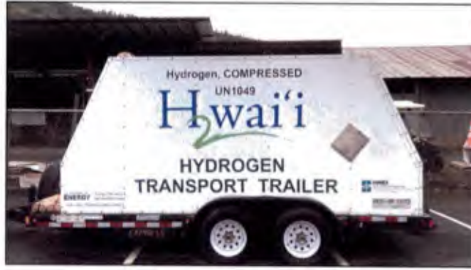
Figure 2.3.3 Hydrogen Transport Trailer.
