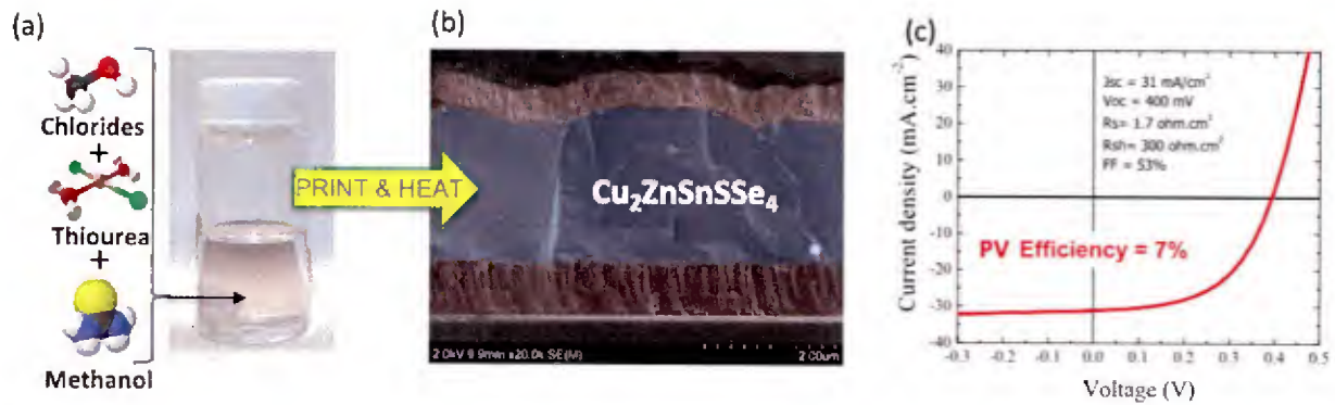
Figure 2.4.1 (a) Picture of a stable molecular ink containing metal chlorides, thiourea and methanol. (b) Scanning electron microscopy cross-sectional view and (c) current-voltage characteristic of a printed CZTSSe solar cell.
