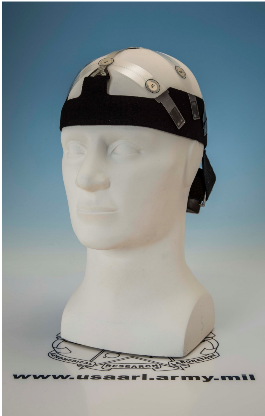
Figure A1. B-Alert X-24 EEG system. This is a wireless, wet electrode system with 20 channels corresponding to scalp locations according to the International 10-20 system. The EEG system provides cognitive state classification algorithms (engagement, distraction, and workload) to be used for data analysis.
