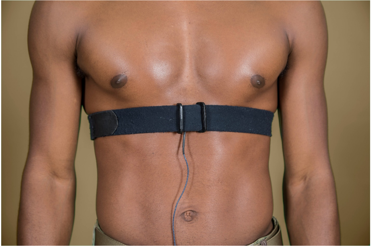
Figure A3. The BioNomadix respiration pneumogram amplifier module was utilized for the collection of respiration data. The transducer strap was placed on the chest or abdomen of the subject and sampled at a rate of 50 Hz.
