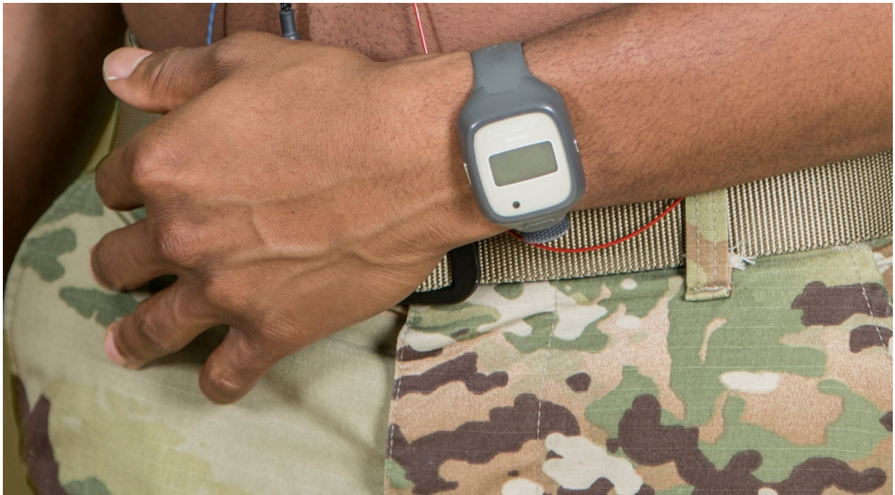
Figure A5. Actiwatch ® activity monitoring system. Subjects were required to wear an Actiwatch ® for the duration of the study in order to ensure he/she was meeting the sleep requirements.
