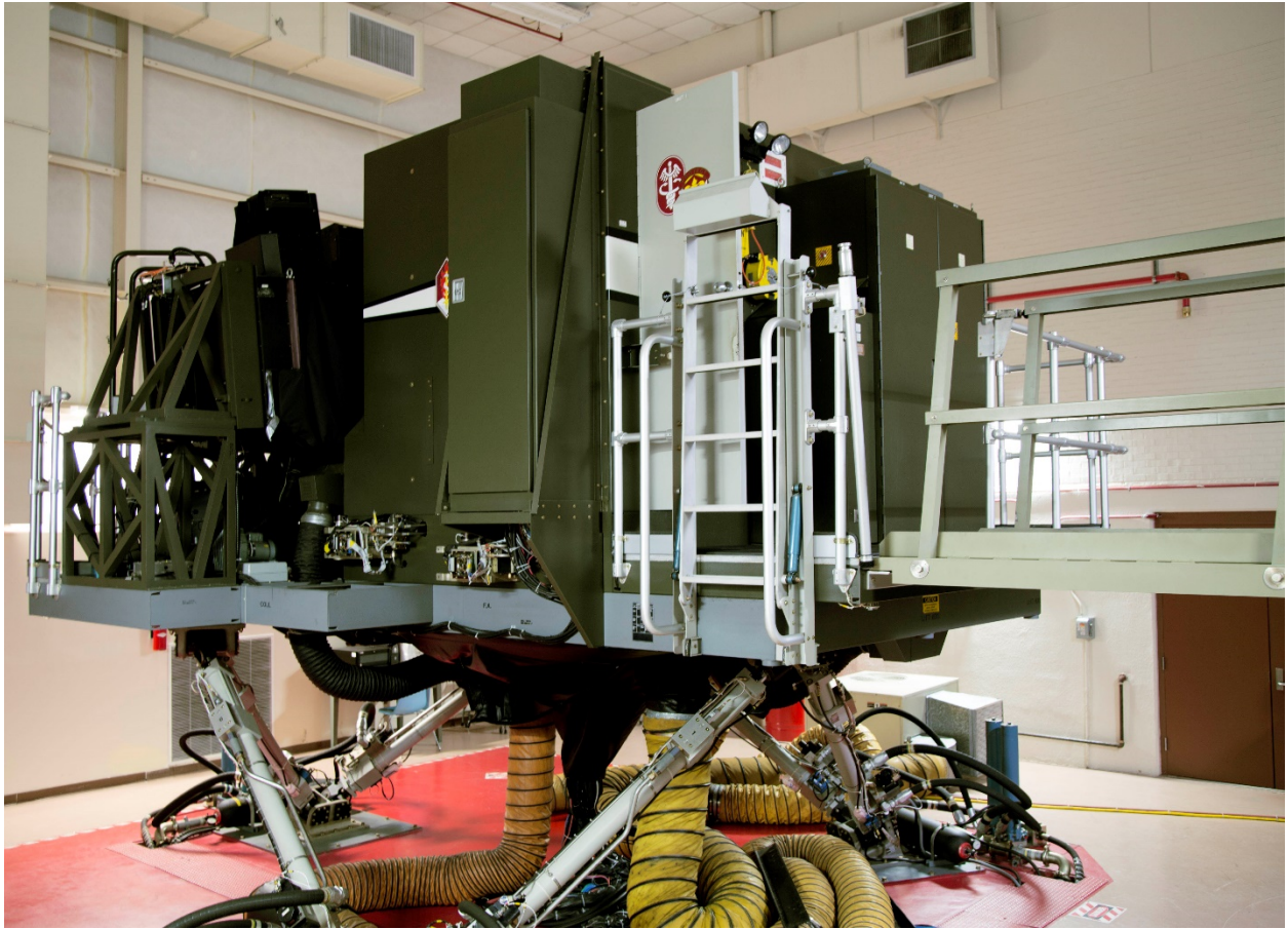
Figure A6. Black Hawk flight simulator consisting of a cockpit, operator station, observer station, and a six-degree-of-freedom-motion system.
