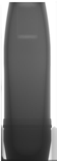
Figure 1. A radiograph of an M1 shell.
