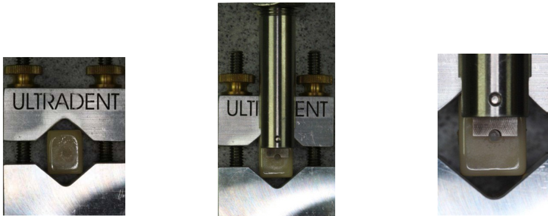
Figure 15: Test base clamp with e.max block (left), crosshead assembly shearing composite button (center) and close-up of crosshead assembly shearing composite button.
