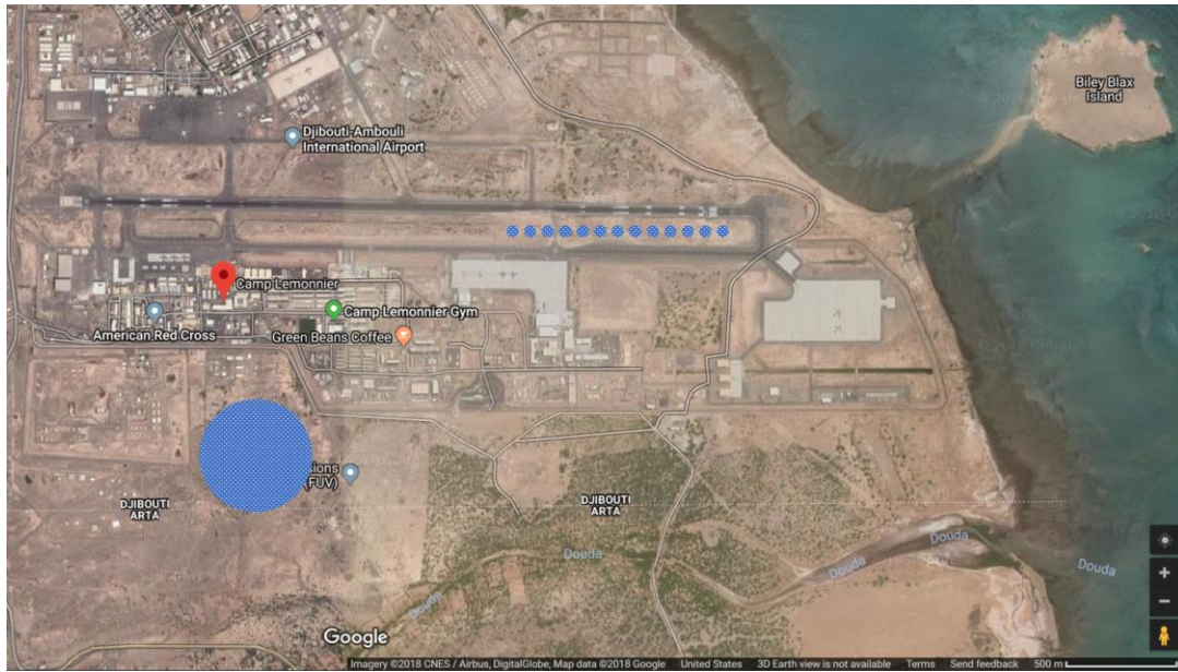
Figure G-4 - Camp Lemonnier in Djibouti, with a notional 500 m diameter space solar receiver and a collection of several 50 m diameter receivers providing equivalent power (shown between runways).
