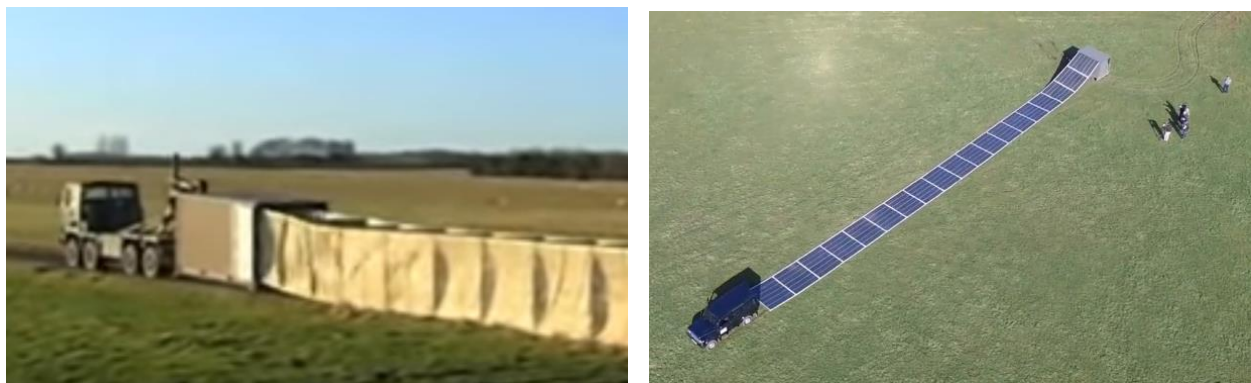
Figure 5-2 - (a) HESCO barrier deployment from a moving truck [61] and (b) Renovagen Rapid Roll T deployment [62].
