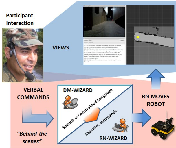
Fig. 1 WoZ setup for our experiment: participant instructs robot with two experimenters standing in for robot capabilities
