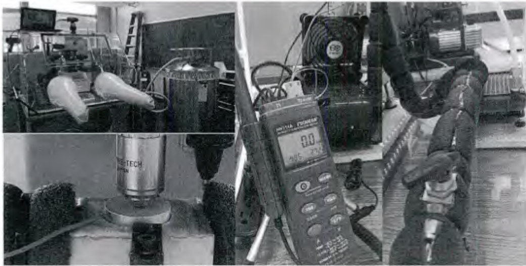
Figure 2 - Cryogenic microindentation apparatus developed for low-temperature testing of materials properties.
