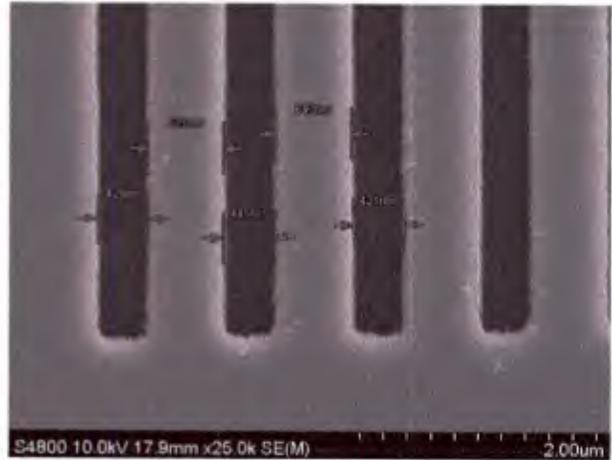
Figure 39: Mesa-Trench 0.6 x 0.4  $\mu\text{m}$
