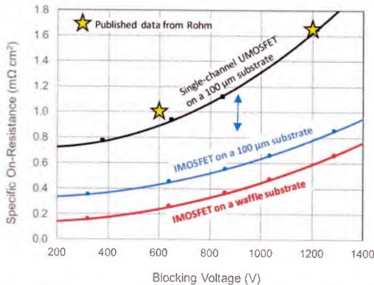
Figure 10: Comparison of simulated  $R_{on,sp}$  of IMOSFETs compared to existing commercial MOSFETs
