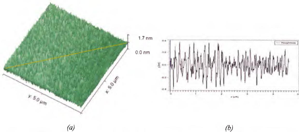
Figure 18: 3D AFM image of across the source and base regions after high energy implantation and activation anneal. The roughness along the cutline (a) is shown in (b). A smooth SiC surface is recovered after the activation anneal process with a surface roughness of  $RQ$  of 0.24 nm.
