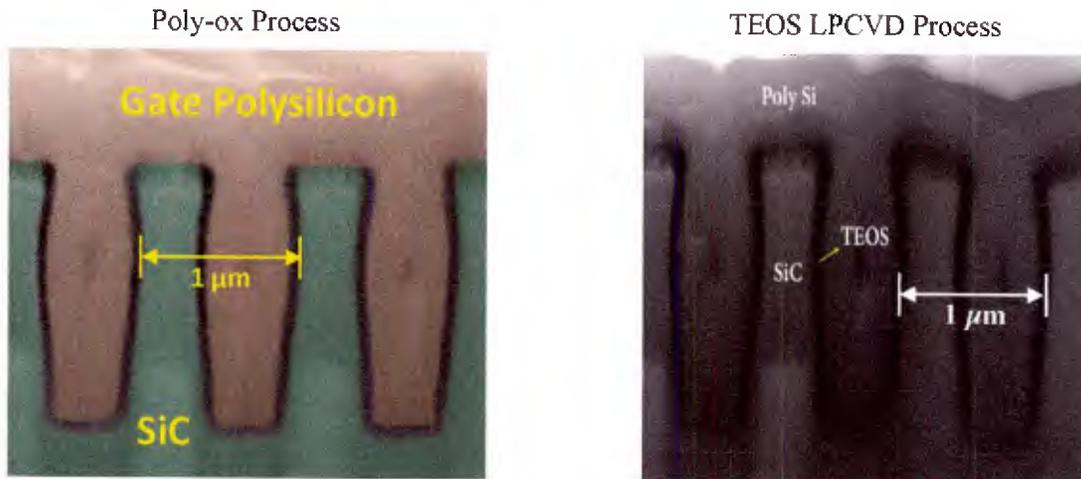
Figure 21: Cross sectional SEM images of the SiC / SiO<sub>2</sub> / polysilicon stack.
