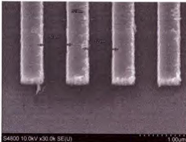
Figure 42: SEM image of Ni mask before etching
