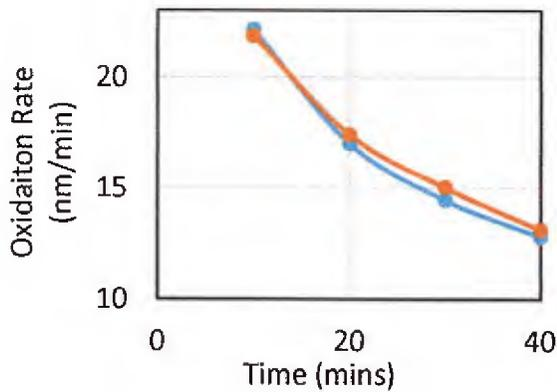
Figure 16: Pyrogenic oxidation of polysilicon at 1100°C.
