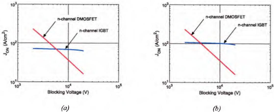
Figure 61: On-current vs. blocking voltage for an  $n$ -channel IGBT and an  $n$ -channel DMOSFET at  $175^\circ\text{C}$  for power dissipation limits of (a)  $200$  W/cm<sup>2</sup> (b)  $300$  W/cm<sup>2</sup>
