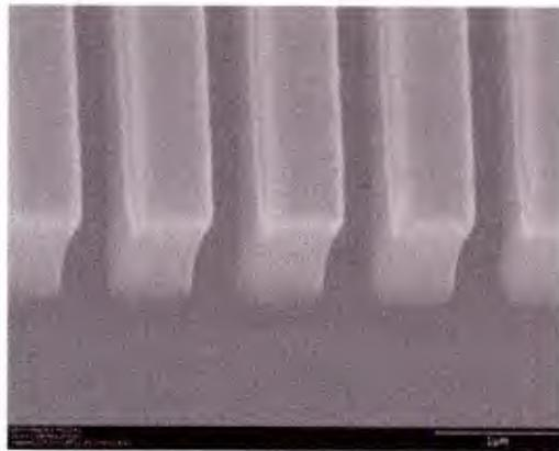
(a) SEM image of the recently developed SiC trench etch in Notre Dame's Oxford Plasma Lab 100 ICP-RIE
