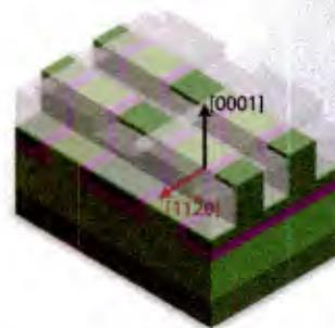
(b) 3D isometric view of the current paths along the sidewall  $\{11\bar{2}0\}$  plane
