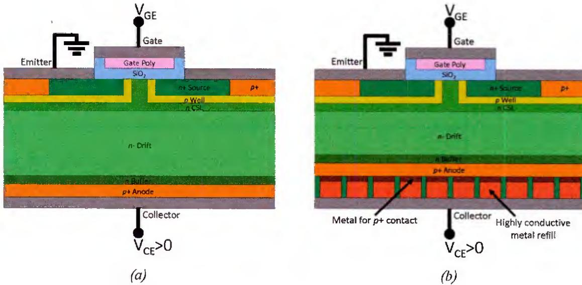
Figure 60: (a) Ultra high voltage  $n$ -channel IGBT without the substrate
