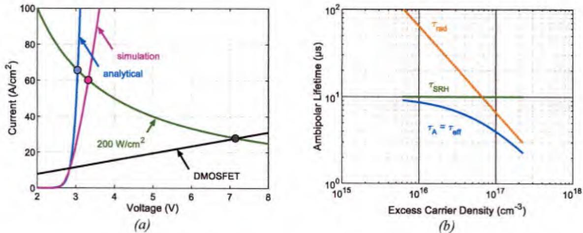
Figure 64: (a) Simulated I-V characteristics of a 12.5 kV n-channel IGBT and a comparable n-channel DMOSFET (b) Ambipolar lifetime as a function of excess carrier density
