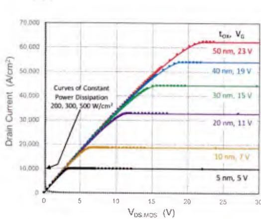
Figure 69. I-V characteristics computed using the bulk-charge equation. Oxide thickness and gate voltage are scaled to keep the oxide field constant at 4 MV/cm ( $Q_g = 1.38 \mu\text{C}/\text{cm}^2$ ).
