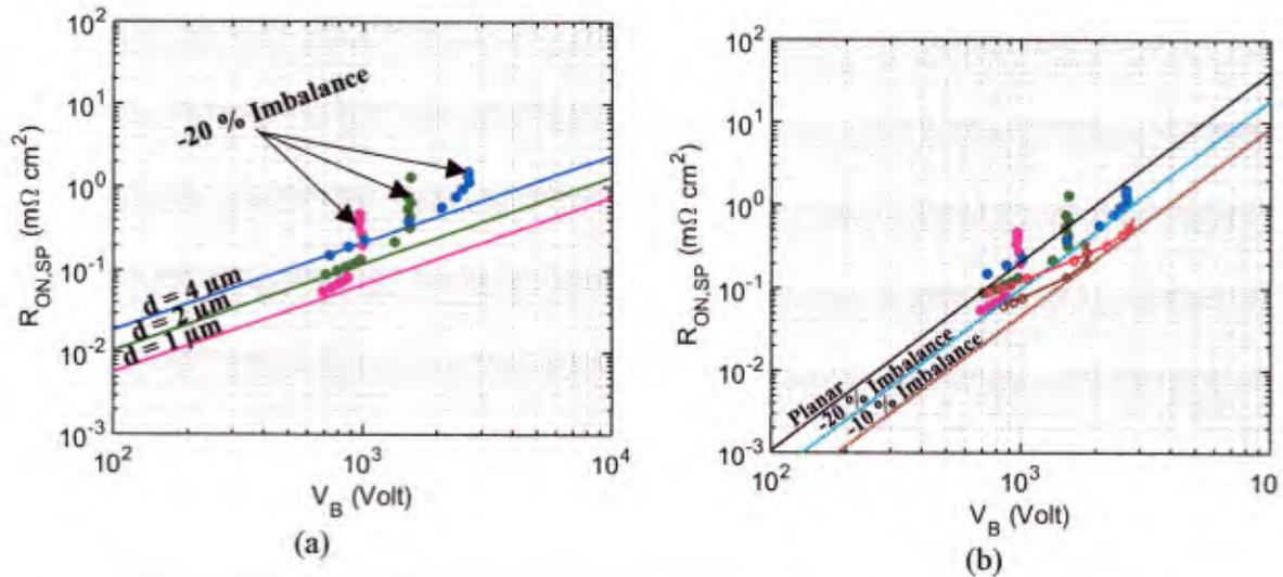
Figure 53: Effect of charge imbalance on superjunction specific on resistance for (a) balanced (lines) and -20% imbalanced (points) SJ devices and pillar widths of 1, 2, and 4  $\mu\text{m}$  (b) -10% (open circles with lines) and -20% (solid circles) imbalanced SJ devices.
