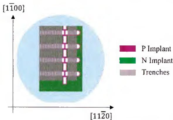
(a) JFET, source and trench finger orientation with respect to the wafer
