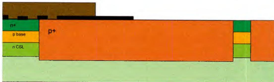
Figure 36: Optical mask to protect active area etch
