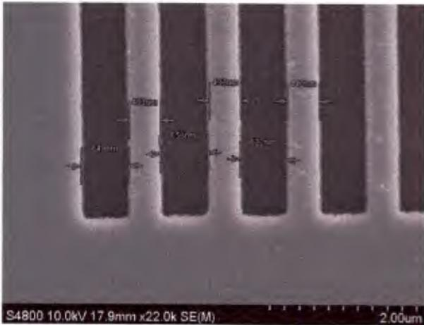
Figure 40: Mesa-Trench 0.4 x 0.6  $\mu\text{m}$
