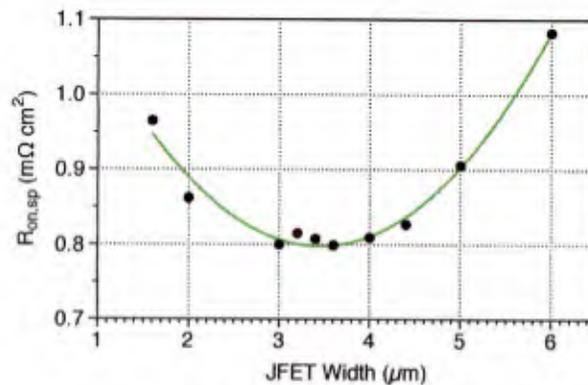
Figure 3: 3D simulation of the 3G-MOSFET specific on-resistance vs. JFET width.
