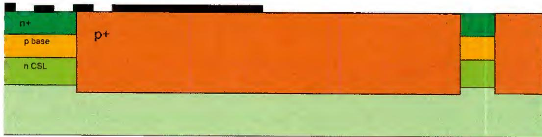
Figure 35: E-beam Ni mask for Gate trench
