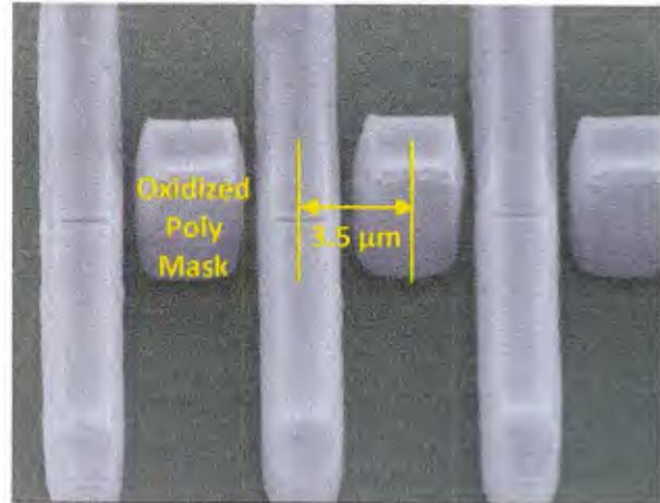
Figure 17: SEM image after polysilicon expansion by oxidation using the self-aligned short-channel process.
