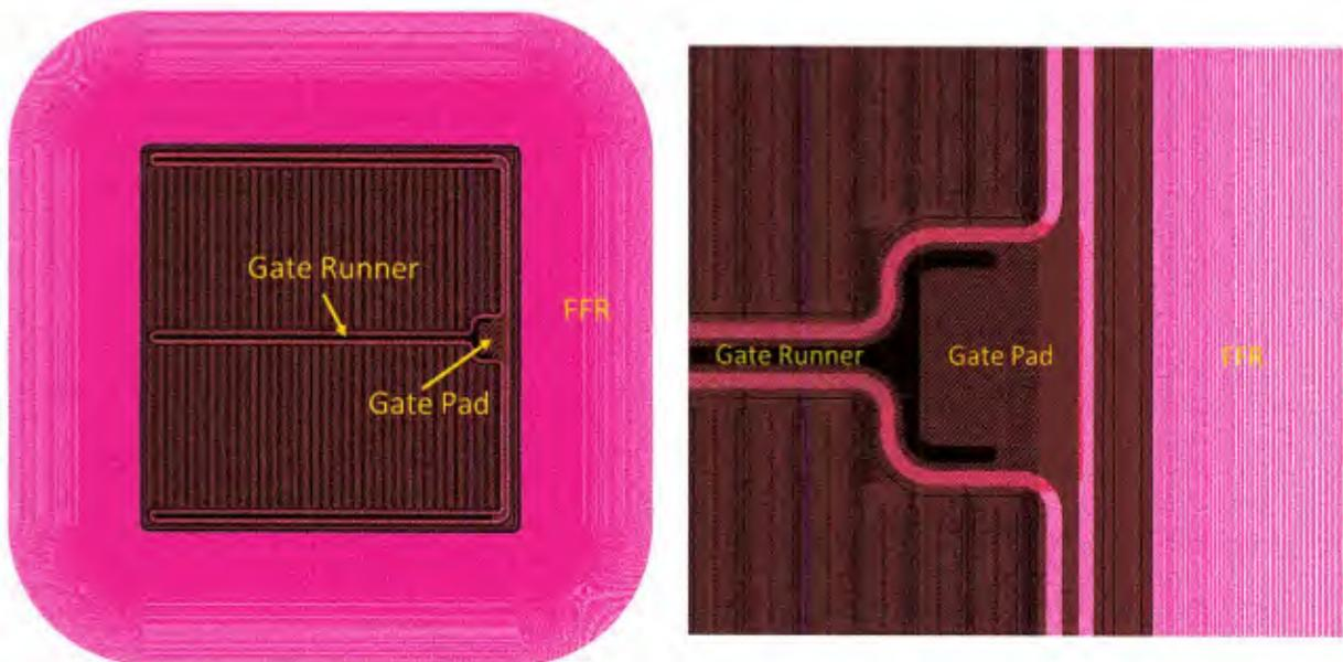
*Figure 65: Sample IGBT from the mask design*
