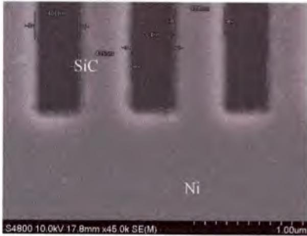
Figure 38: Mesa-Trench 0.4 x 0.4  $\mu\text{m}$
