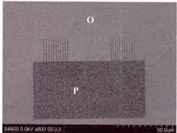
(b) Top view of etched oxide
