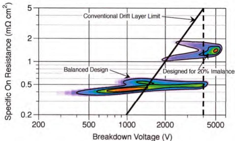
Figure 58: Contour plots of  $R_{on,sp}$  vs.  $V_{BR}$  for balanced SJ designs and designs optimized for 20% charge imbalance and a target blocking voltage of 4 kV. The contours enclose 10%, 50%, and 90% of the devices. The lower contour plot assumes a balanced nominal design, and the upper contour plot is for a SJ design optimized for 20% imbalance.
