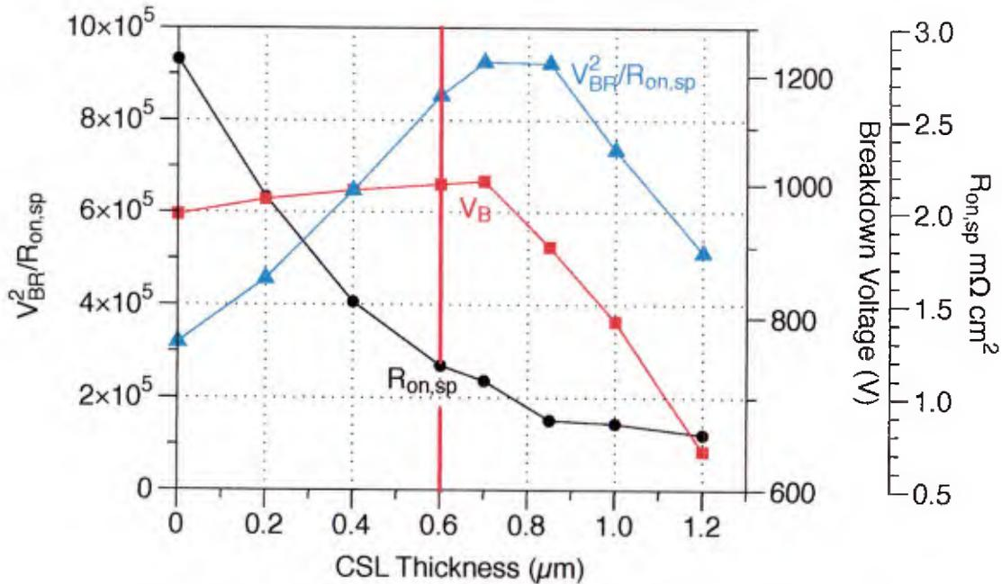
Figure 5: Performance vs CSL thickness for a JFET width of  $2.0 \mu\text{m}$ . The red line is the selected design point.
