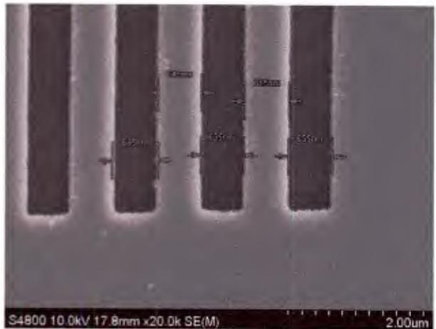
Figure 41: Mesa-Trench 0.6 x 0.6  $\mu\text{m}$
