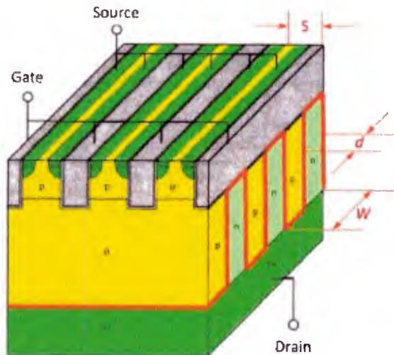
Figure 51: A superjunction drift region, as implemented in a silicon UMOFET.
