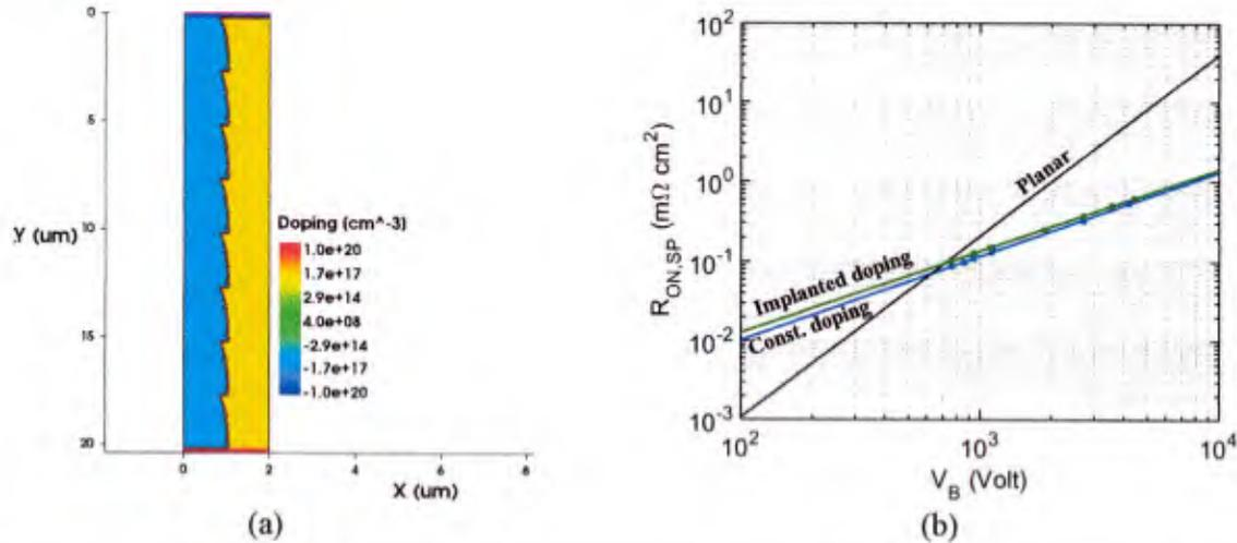
Figure 54: (a) Simulated multicycle epi-implant SJ drift layer (b)  $R_{on,sp}$  vs.  $V_b$  for a conventional drift region, an ideal uniformly-doped SJ, and a multicycle epi-implant SJ.
