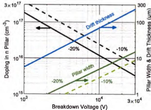
Figure 56: Optimum design parameters for SJ's in 4H-SiC as a function of  $V_{BR}$  for charge imbalances of -20% (solid lines) and -10% (dashed lines).
