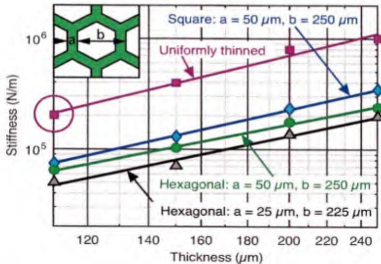
Figure 47: ANSYS simulation results of patterned and unpatterned 4H-SiC substrates of different dimensions. The circle represents the uniformly-thinned 110  $\mu\text{m}$  substrate reported by Infineon as their production process. Waffle substrates on a wafer thinned to 200  $\mu\text{m}$  would exhibit comparable stiffness.
