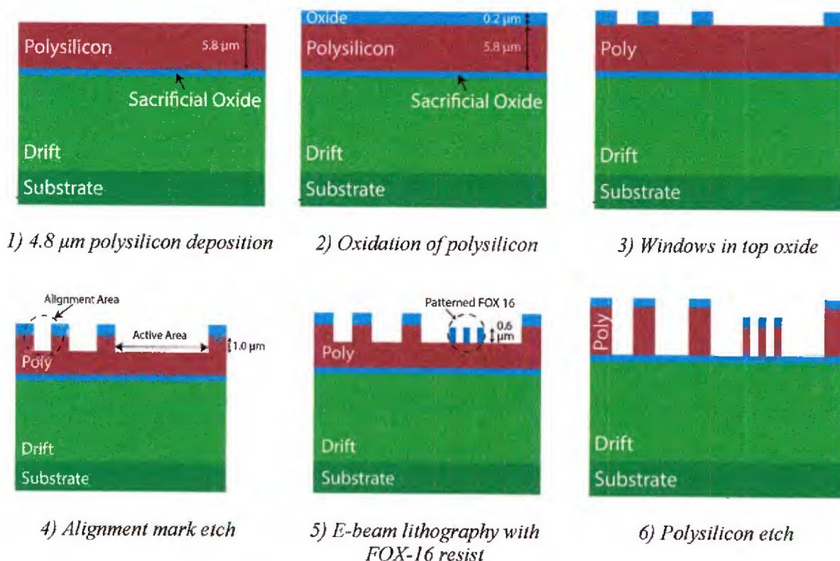
Figure 14: Oxide-only polysilicon implant mask etch process sequence.
