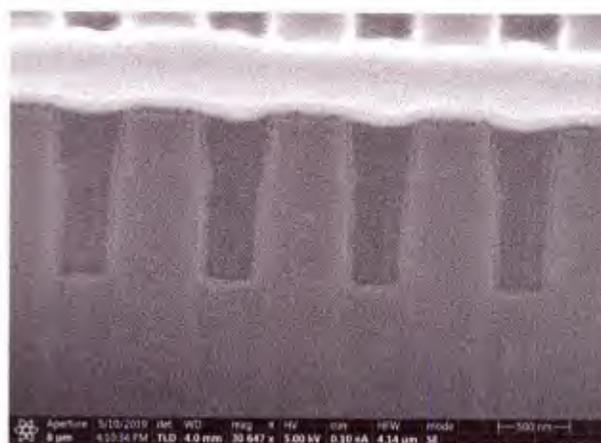
Figure 44: FIB cross-section of poly filled trenches
