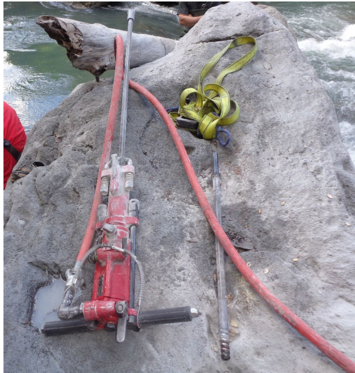
Figure 24. AIRREX Panther rock drill with 4-ft shaft.
