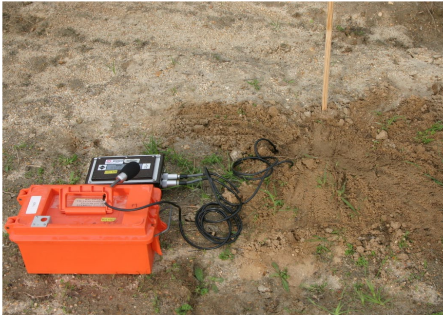
Figure 32. Typical Miniseis unit deployed for blast monitoring.
