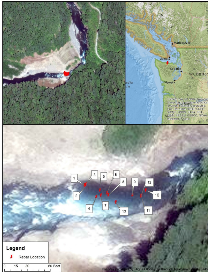
Figure 3. Surveyed metal debris locations at ELD site (survey limited to left portion of channel).
