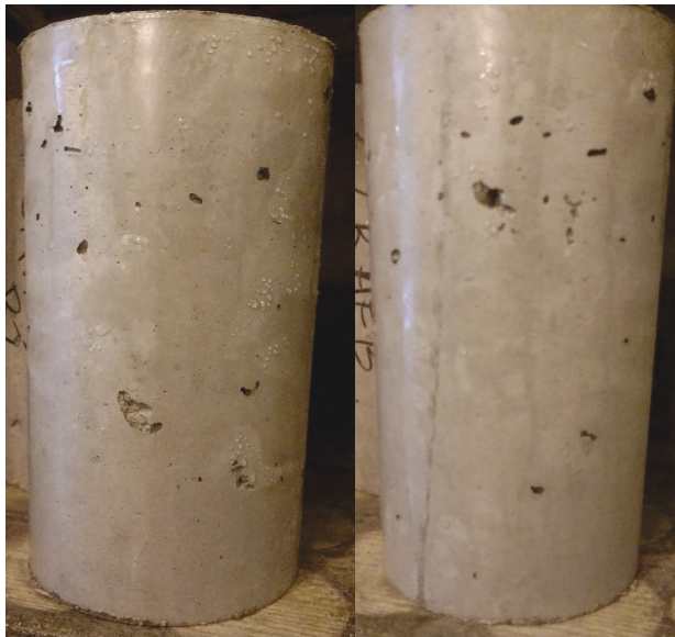
Figure 8. Specimen photos illustrating unclosed holes.
