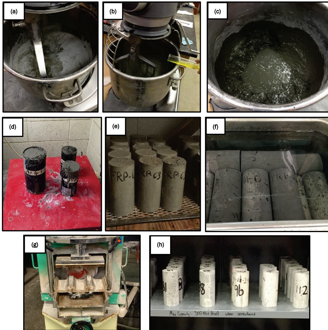
Figure 1. (a) Mixing dry materials and water, (b) adding admixture, (c) finished mixture, (d) vibration table, (e) specimens in curing room, (f) specimens in water bath, (g) end grinding, and (h) shelved specimens awaiting testing.
