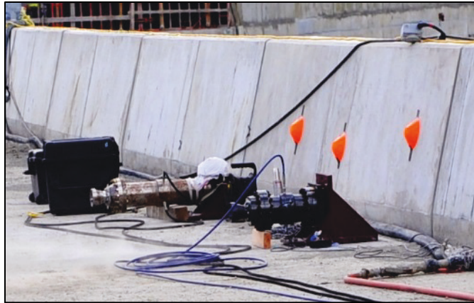
Figure 2. Cold Gas Thrusters mounted onto Portugues Dam.
