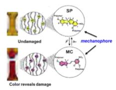
**Figure 1.** First demonstration of mechanoresponsiveness in solid-state materials
