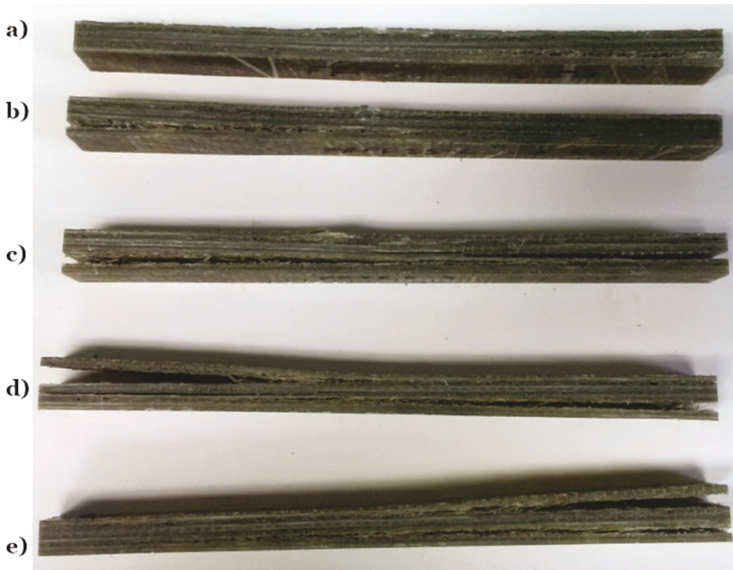
Figure 19. FRP panel specimens after flexural testing at various temperatures: a) 73; b) 25; c) 0; d) -25; e) -40 °F.
