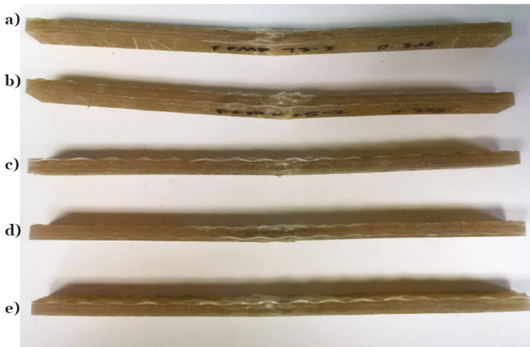
Figure 17. FFM specimens after flexural testing at various temperatures: a) 73; b) 25; c) 0; d) -25; e) -40 °F.
