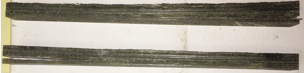
Figure 22. A comparison of the delamination characteristics of the FRP specimens subject to flexural testing: upper specimen was subject to single load-to-failure and shows distinct glass fibers between delaminated layers at the right end; the lower specimen was subject to cyclic flexural testing wherein the glass fibers were worn from between the layers as evident at the left end of the specimen.
