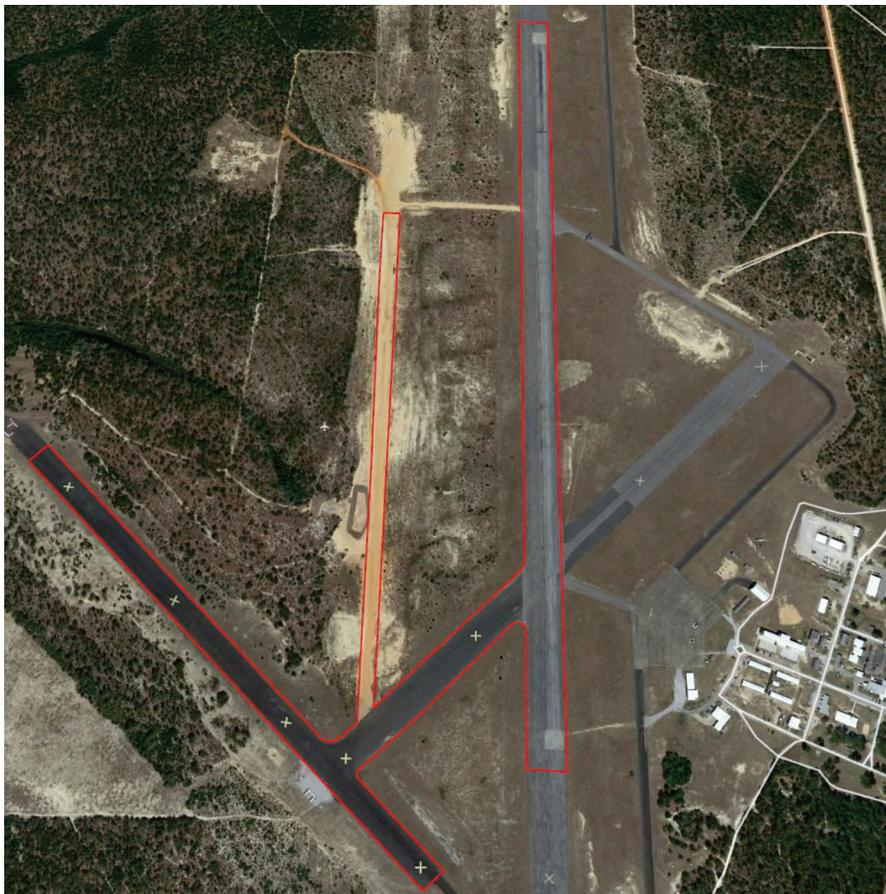
Four pavement surface types were tested at the Camp Rudder airfield: sand-asphalt, dirt, main runway asphalt, and concrete pad. These surfaces provide a varying roughness profile in order to test the EO and LiDAR-based measurement techniques.
