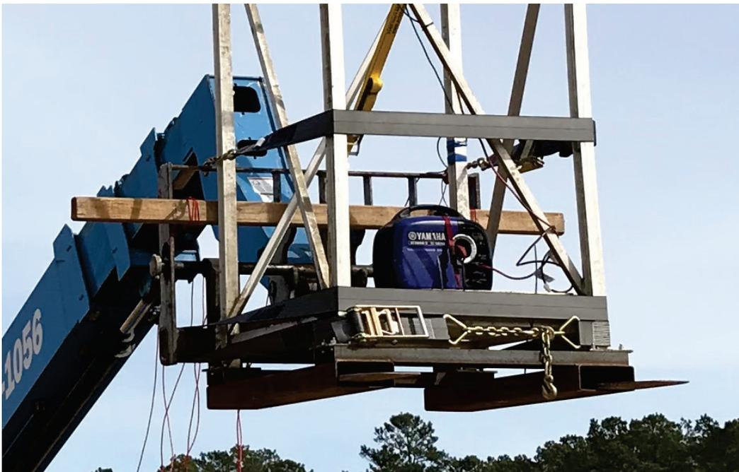
Once the tower was securely fastened to the telehandler, the telehandler was lifted and then lowered at an angle to allow for laser mounting (Figure 10). In this position, the laser system can be activated and instrumented for use during data collection. Once laser system setup was complete, the tower was straightened and held at a low boom height to allow for safe telehandler travel to the survey area.
