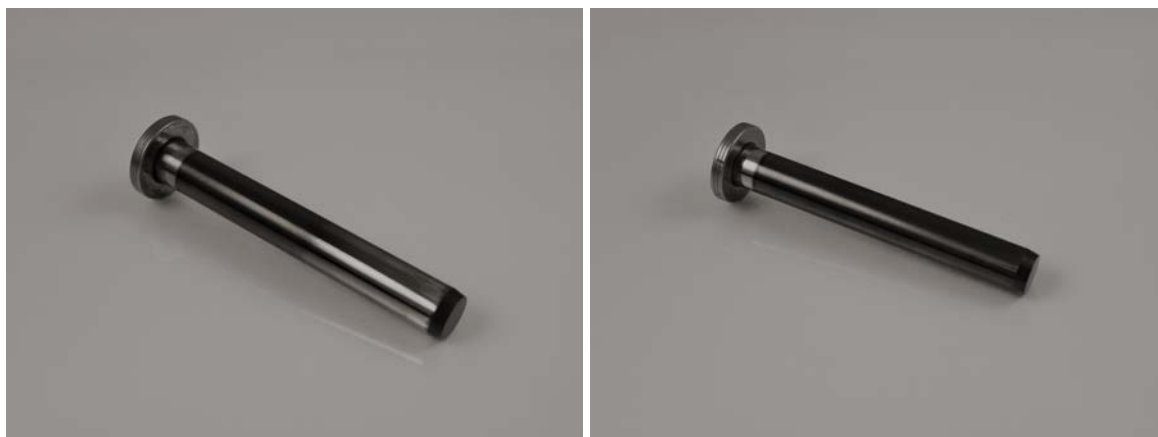
Figure 22. C7 HEUI Injector Plunger (CYL#1 shown left, NEW shown right)
