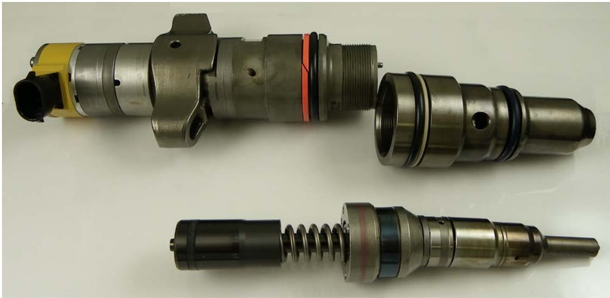
Figure 20. Caterpillar C7 HEUI Injector – Barrel Assembly Removal
