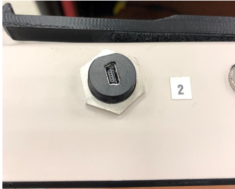
Figure 16. Fix with a metal nut to the pushed-in (broken) USB connector with a metal nut.
