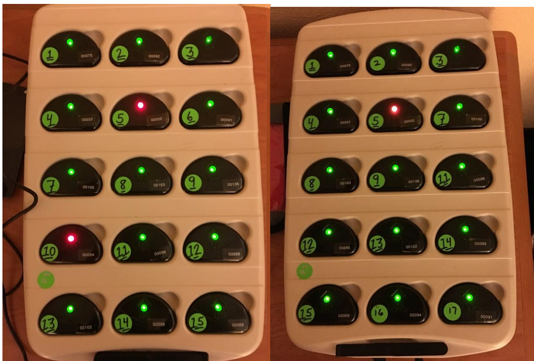
Figure 14. Hubs charging in charging dock after 15 hours of charging. On left – Day 1; two hubs with red lights and on right – Day 2; one hub with red light on.
