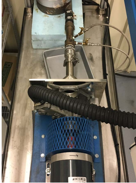
Figure 3. Pump Connection to Calibrated Flow Meter
