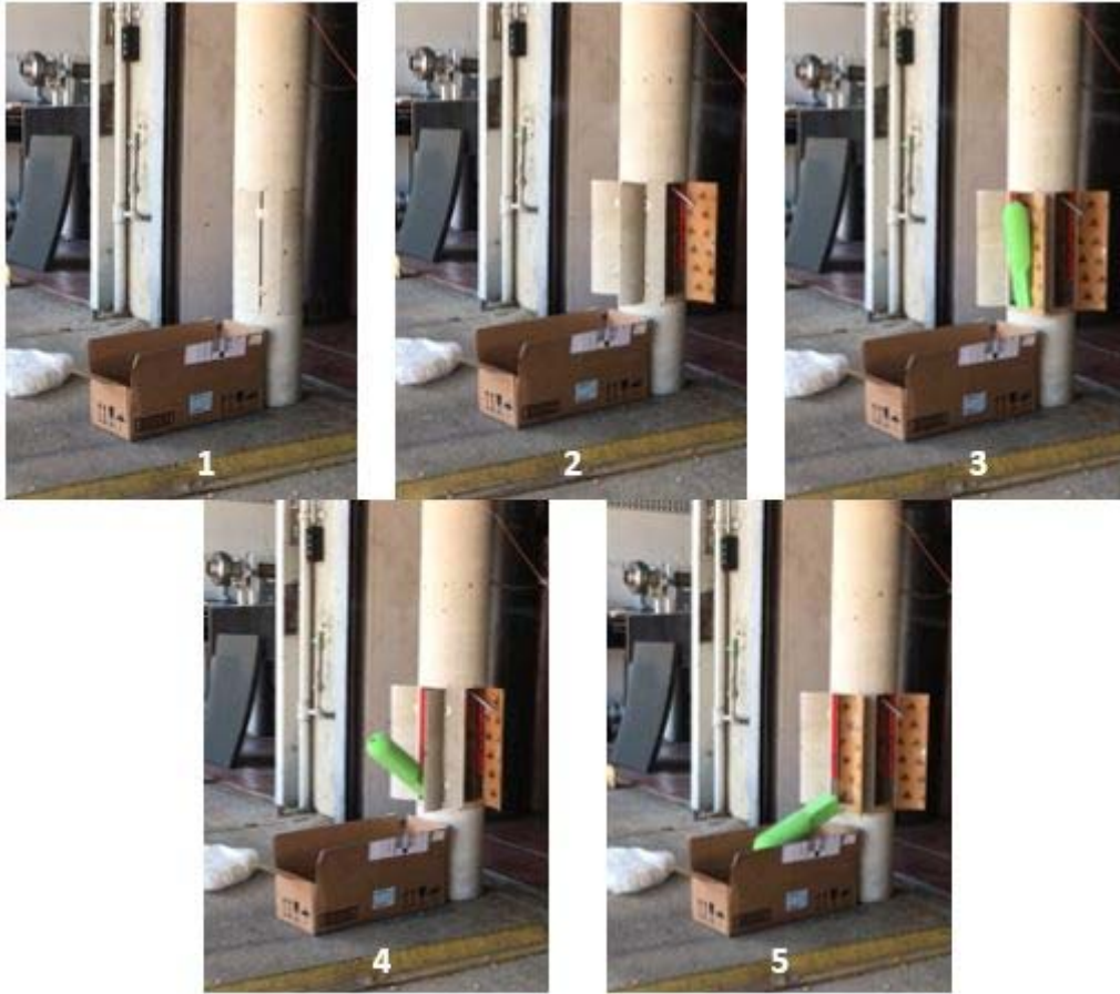
Figure 43. GM deployment during ground test.
