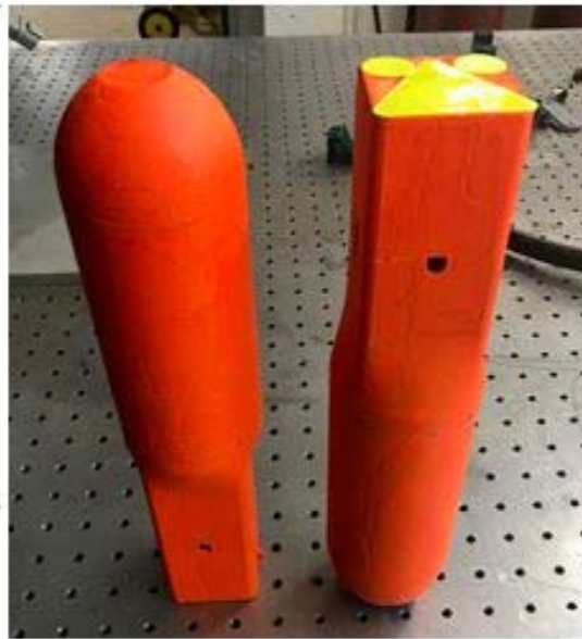
Figure 56. GMs with fluorescent paint and aft end reflectors.
