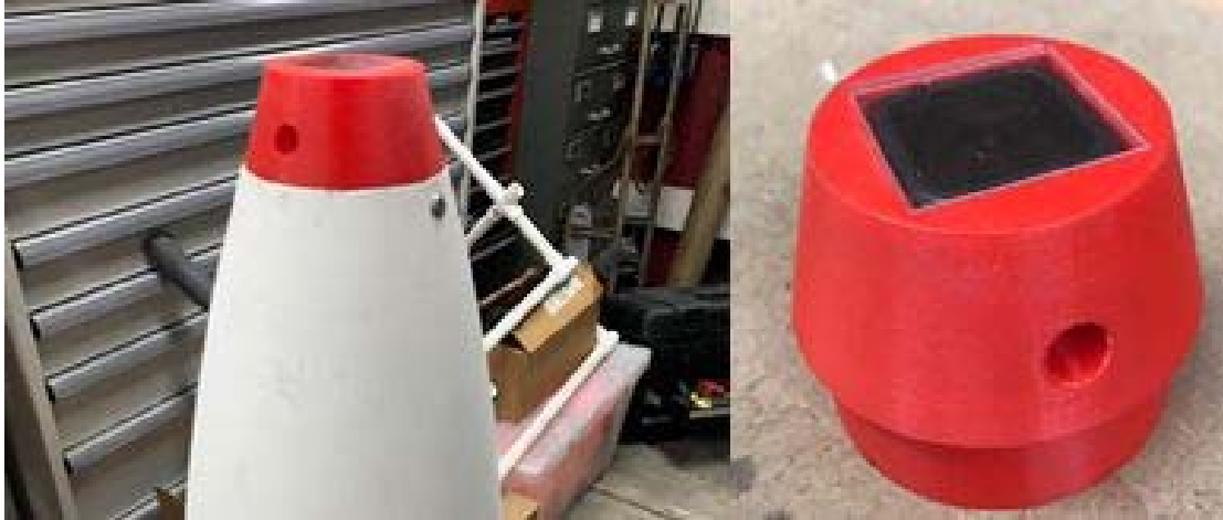
Figure 57. Nose cone camera housing for GoPro Hero 5 Session.
