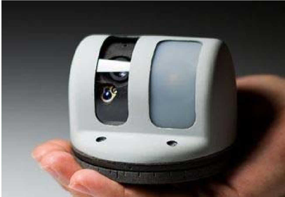
Figure 55. Lockheed Martin Perceptor Dual Sensor gimbal. Source: [47]
