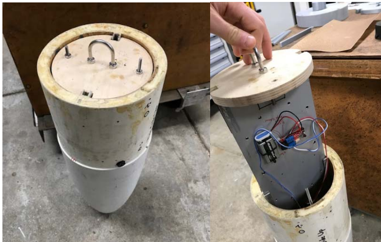
Figure 10. Sliding electronics tray in nose cone.
