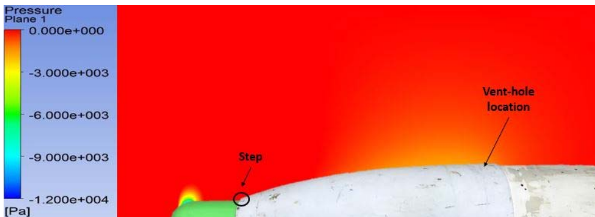
Figure 15. CFD relative pressure solution from -1.2 \times 10^4 Pa to 0 Pa.
