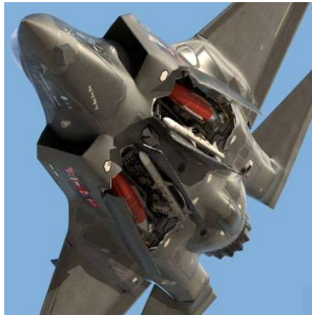
Figure 21. Outward opening bomb bay doors on the Lockheed Martin F-35. Source: [20]
