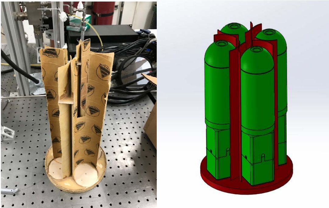
Figure 20. GM bay housing for four GMs.
