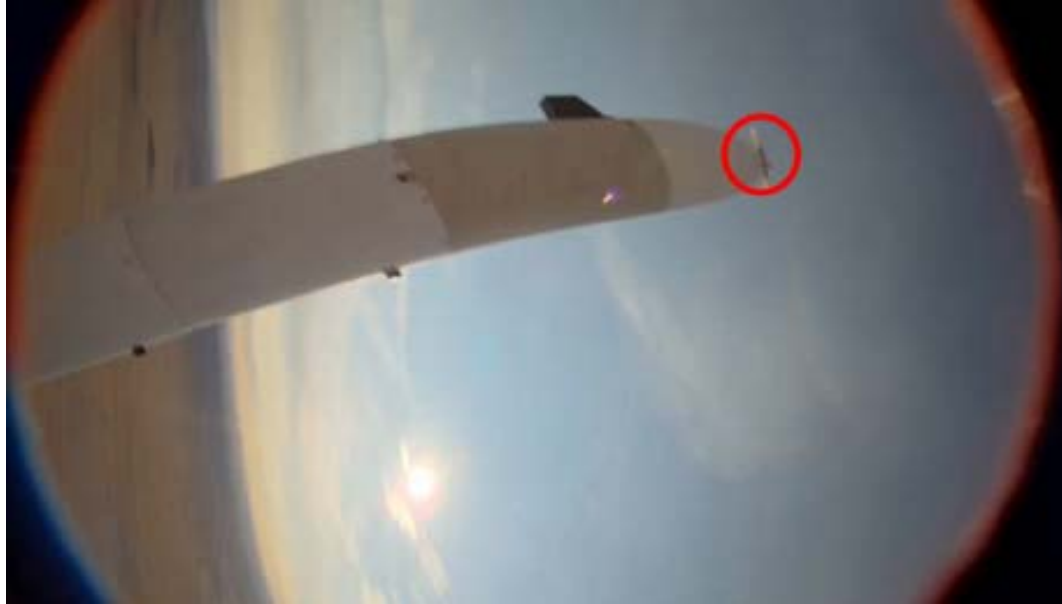
Figure 12. GM lower-half remaining in nose cone, as seen by GM upper-half.
