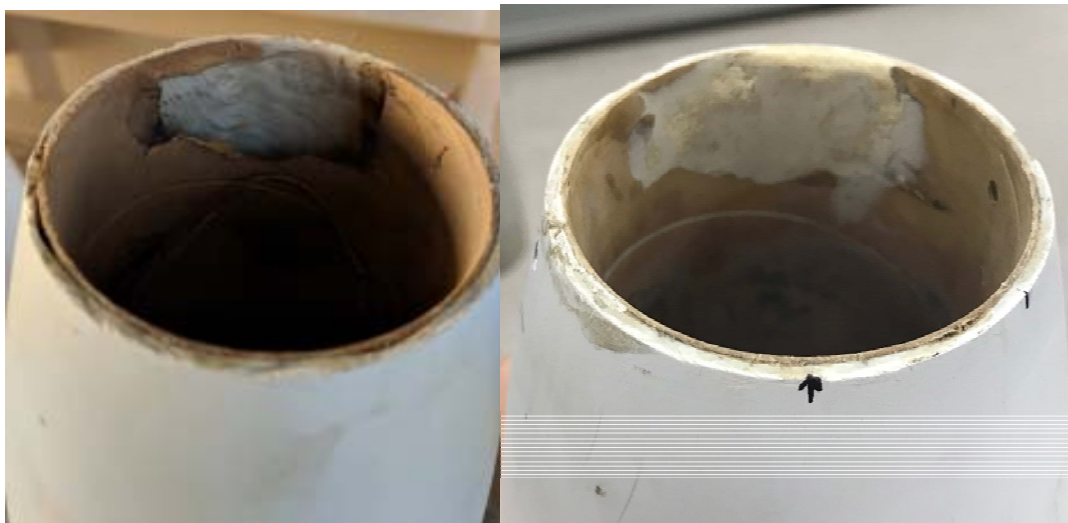
Figure 16. Nose cone tubing damage and repair.
