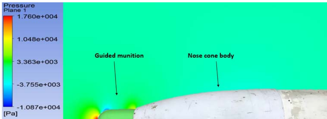
Figure 14. CFD global pressure solution of nose cone with GM protruding.
