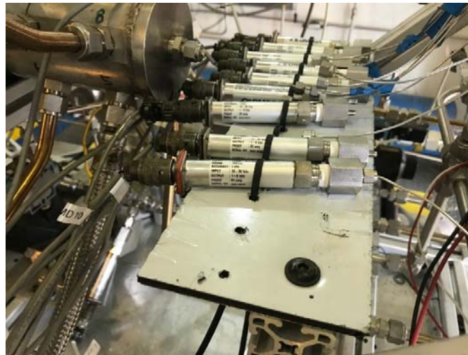
Figure 37. Pressure transducers from RDE test cell.
