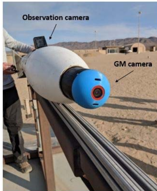
Figure 8. Single GM deployment from nose cone.
