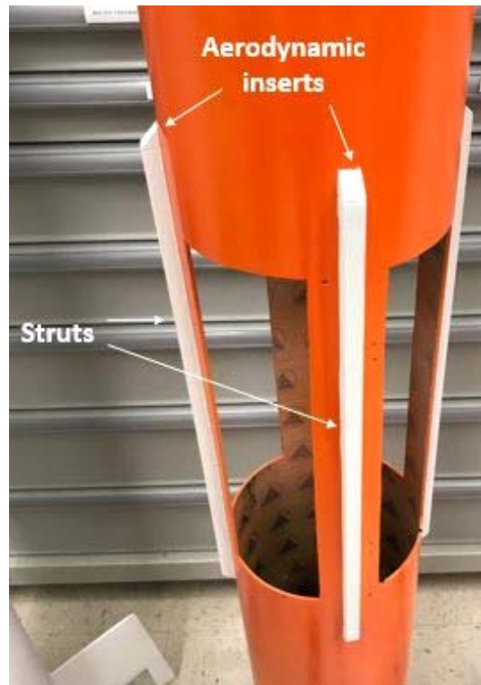
Figure 53. Aluminum strut fortifications added to GM bay.
