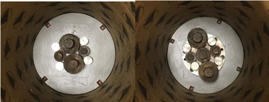
Figure 35. Incrementally adding weights to piston head.
