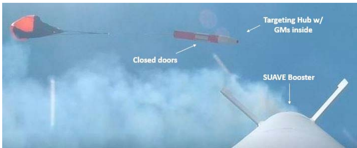
Figure 59. Upper stage with closed doors as seen from lower stage.
