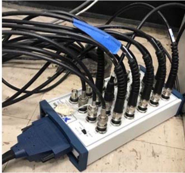
Figure 15. NI BNC-2111 Instrumented with TC2 BNC Wires
