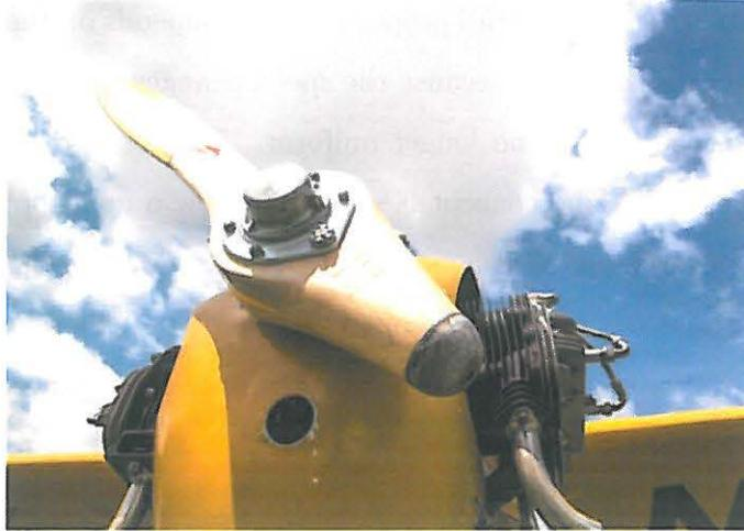
Figure 2-5: Everel propeller mounted on a J-2 Cub aircraft
