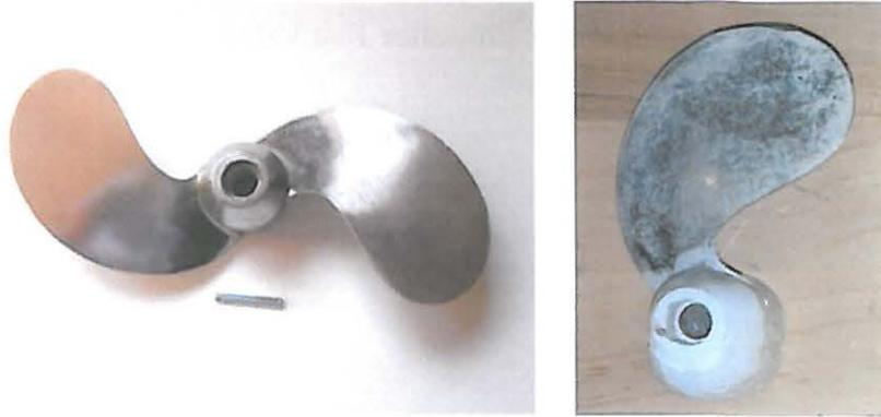
Figure 4-17: Aluminum propeller used for 1-blade propeller testing
