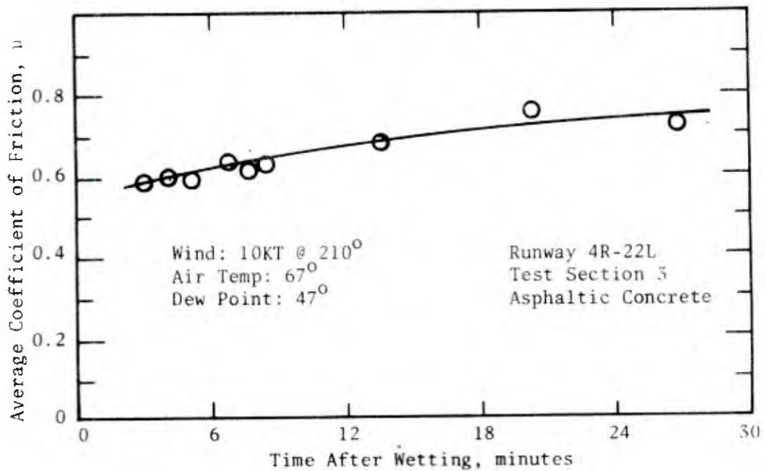
FIGURE 14. AVERAGE FRICTION COEFFICIENT VERSUS TIME AFTER WETTING, USNAS LOS ALAMITOS, CALIFORNIA
