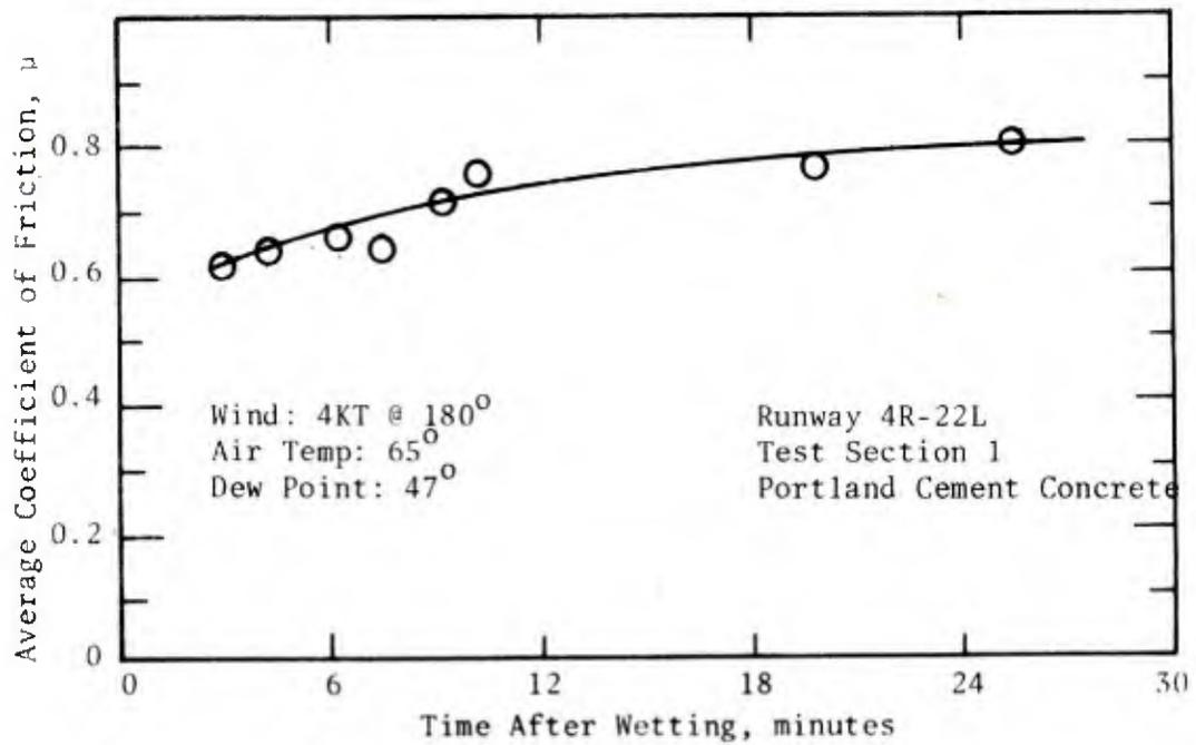
FIGURE 13. AVERAGE FRICTION COEFFICIENT VERSUS TIME AFTER WETTING, USNAS LOS ALAMITOS, CALIFORNIA
