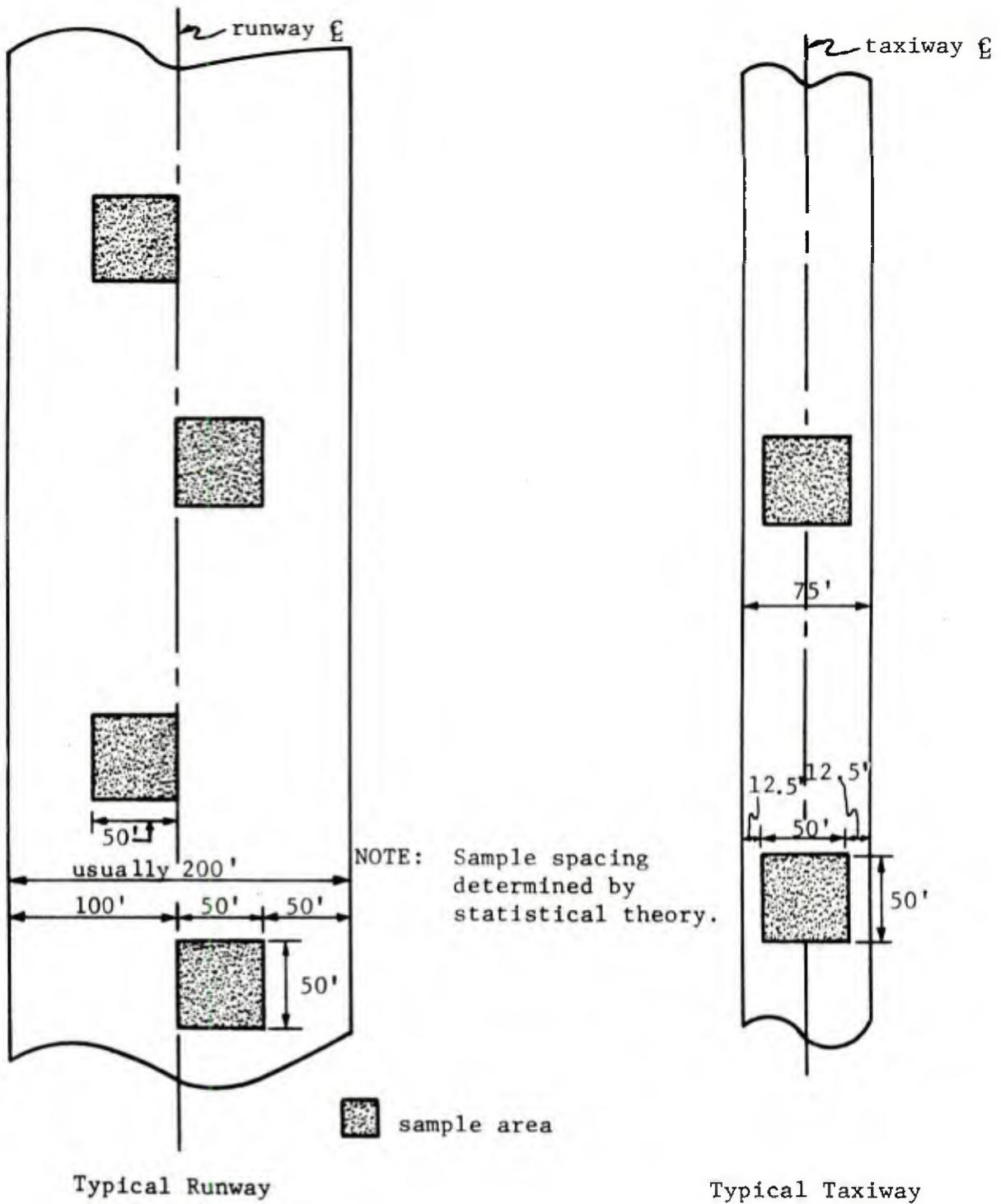
Figure C-2. Asphaltic concrete sample areas.
