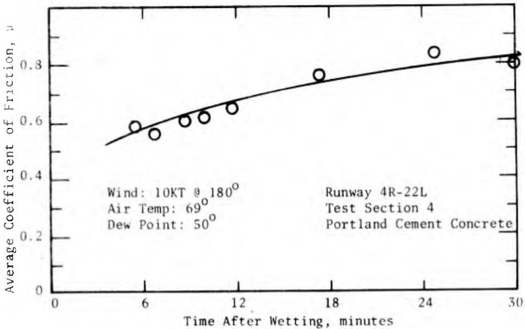
FIGURE 15. AVERAGE FRICTION COEFFICIENT VERSUS TIME AFTER WETTING, USNAS LOS ALAMITOS, CALIFORNIA
