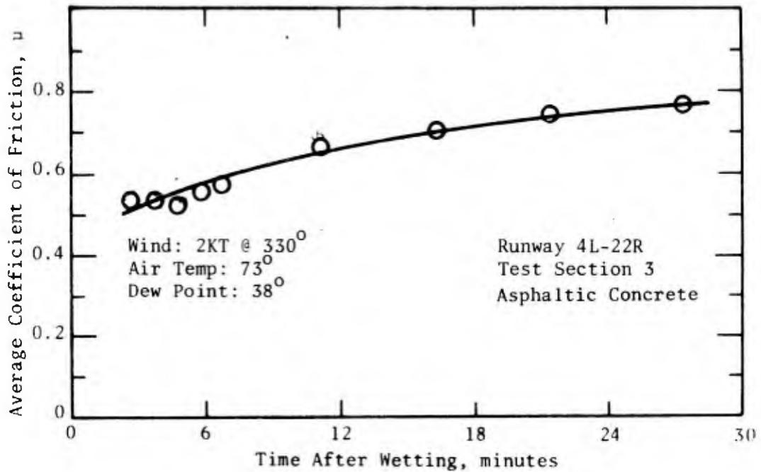
FIGURE 17. AVERAGE FRICTION COEFFICIENT VERSUS TIME AFTER WETTING, USNAS LOS ALAMITOS, CALIFORNIA
