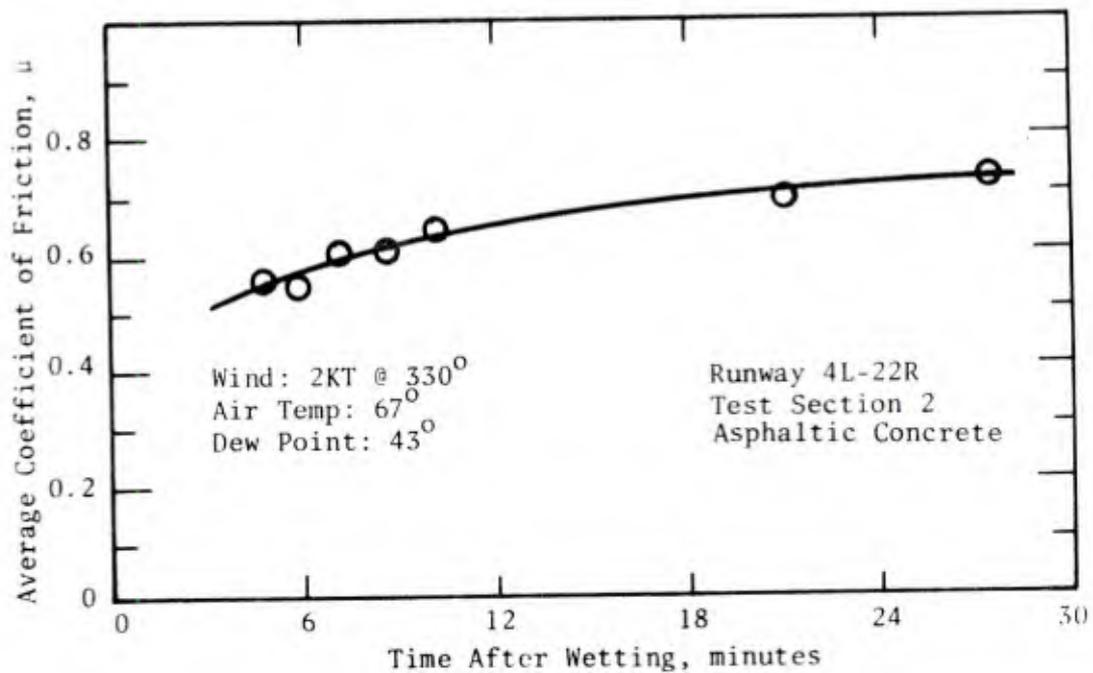
FIGURE 16. AVERAGE FRICTION COEFFICIENT VERSUS TIME AFTER WETTING, USNAS LOS ALAMITOS, CALIFORNIA
