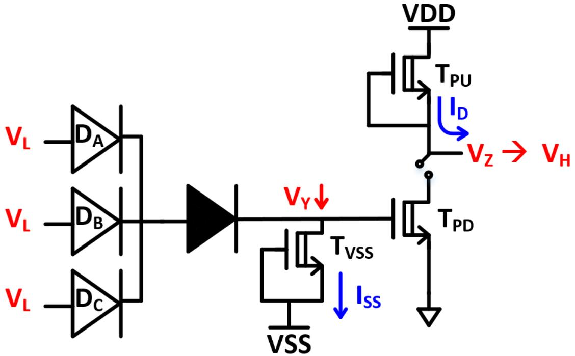
Figure 3.2: SDFL NOR3 Logic Gate with Low Inputs
