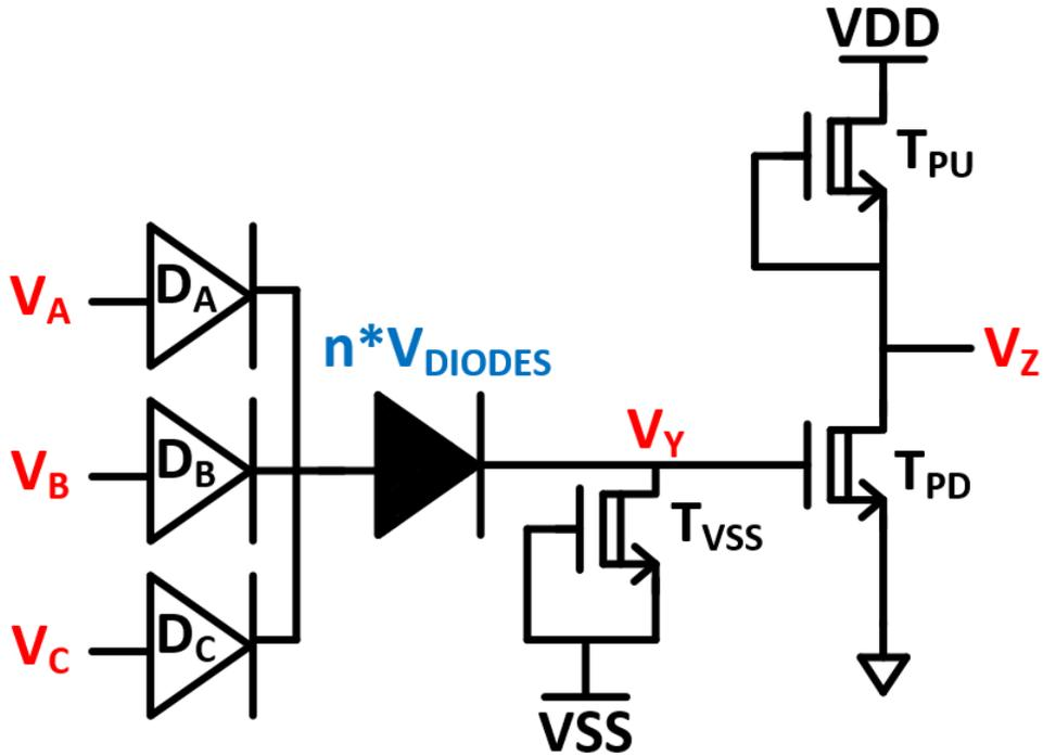
Figure 3.1: SDFL NOR3 Logic Gate
