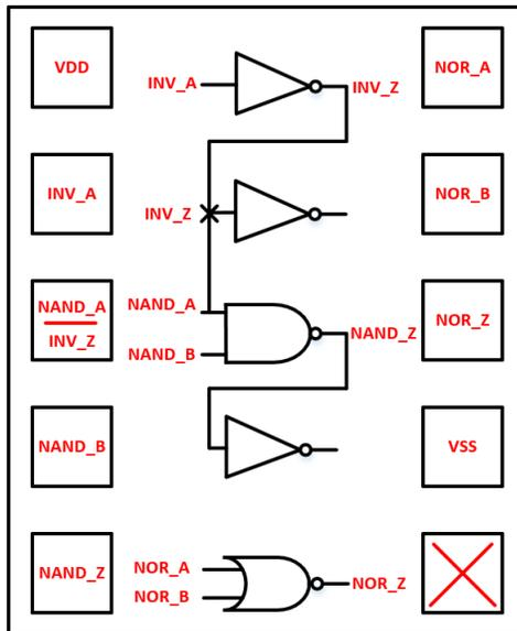
Figure 5.3: Gate Structure of A1/A3 Logic Banks
