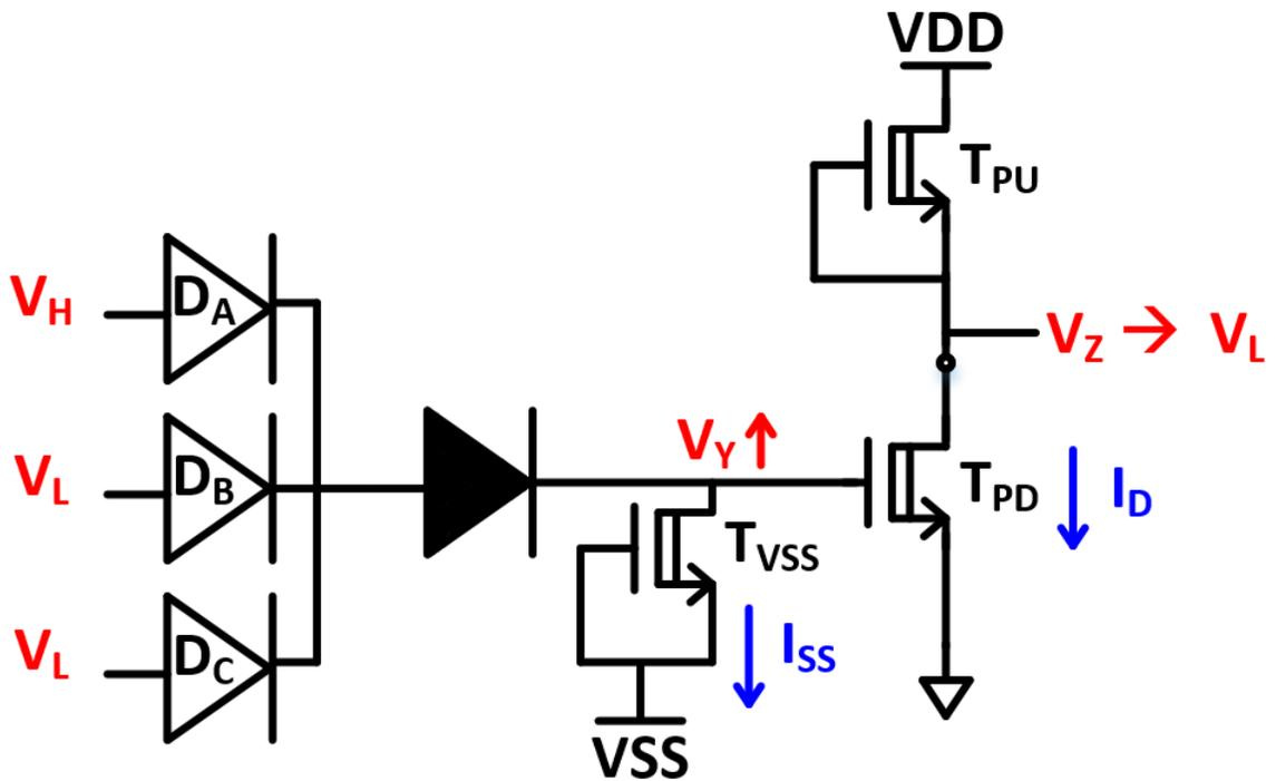
Figure 3.3: SDFL NOR3 Logic Gate with One High Input
