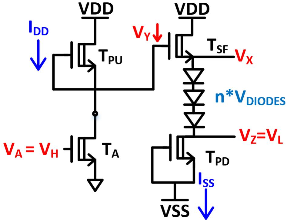
Figure 4.3: BFL INV Gate with Logic High Input
