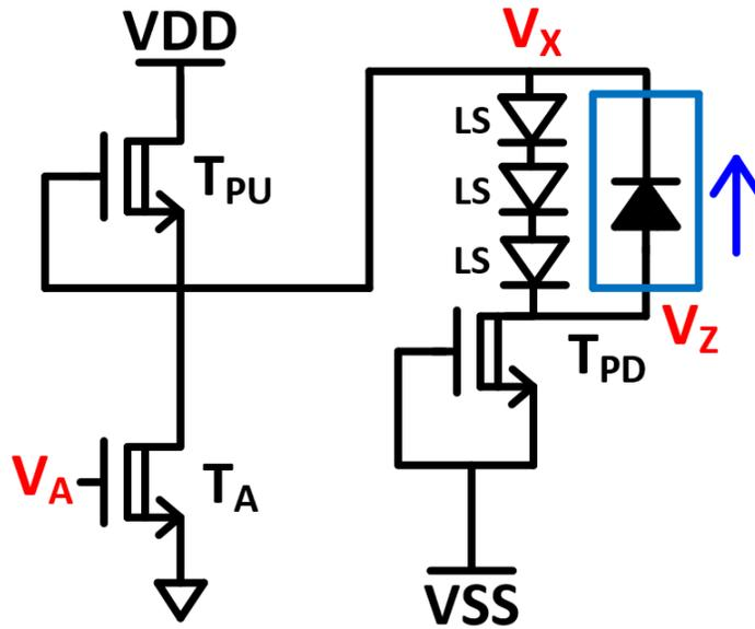
Figure 3.7: CDFL INV Gate with Capacitive Feedforward Reverse Biased Diode
