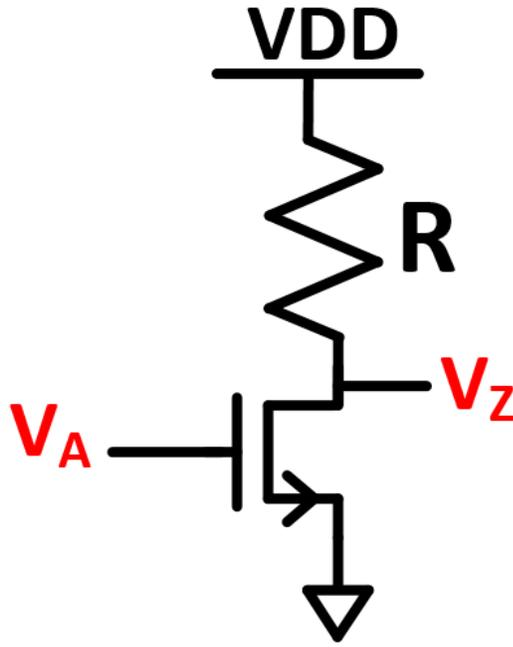
Figure 2.3: N-Channel Only Inverter with Pull Up Resistor
