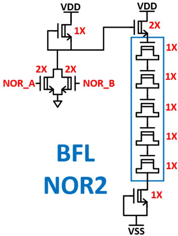
Figure 4.6: BFL NOR2 with Diode Connected Level Shifting
