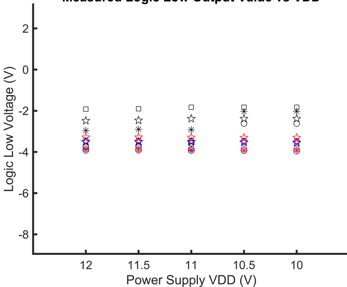
Figure A.7: Measured Logic Low Value
