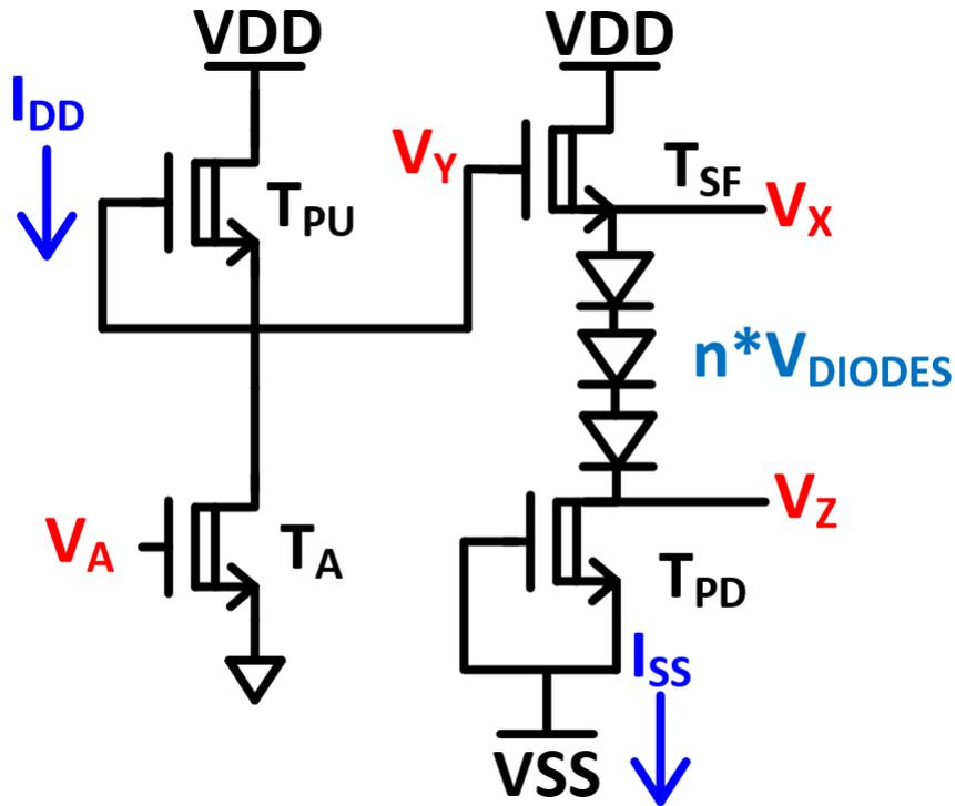
Figure 3.9: BFL INV Gate using Source Follower Buffer
