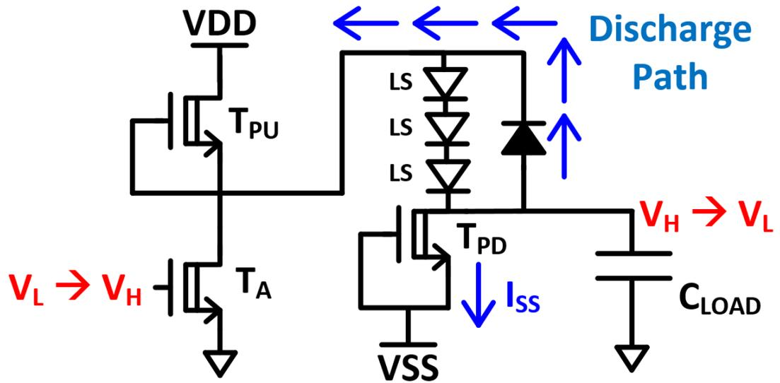
Figure 3.8: CDFL INV Gate with Output Discharge through Feedforward Diode
