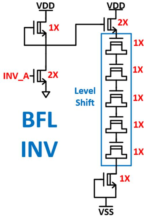
Figure 4.5: BFL Inverter with Diode Connected Level Shifting
