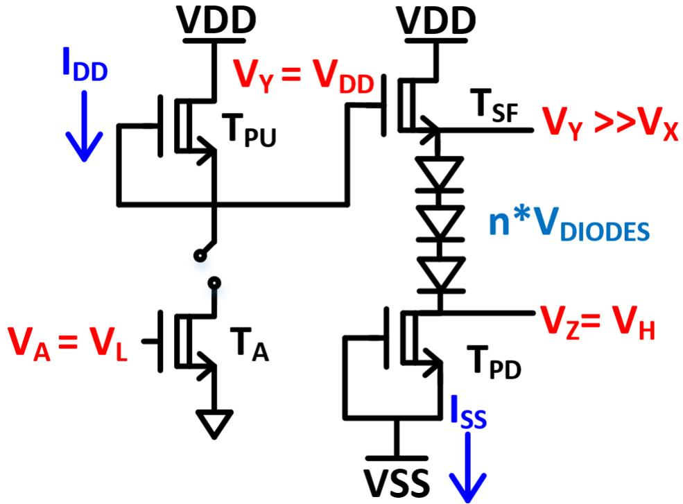
Figure 4.2: BFL INV Gate with Logic Low Input
