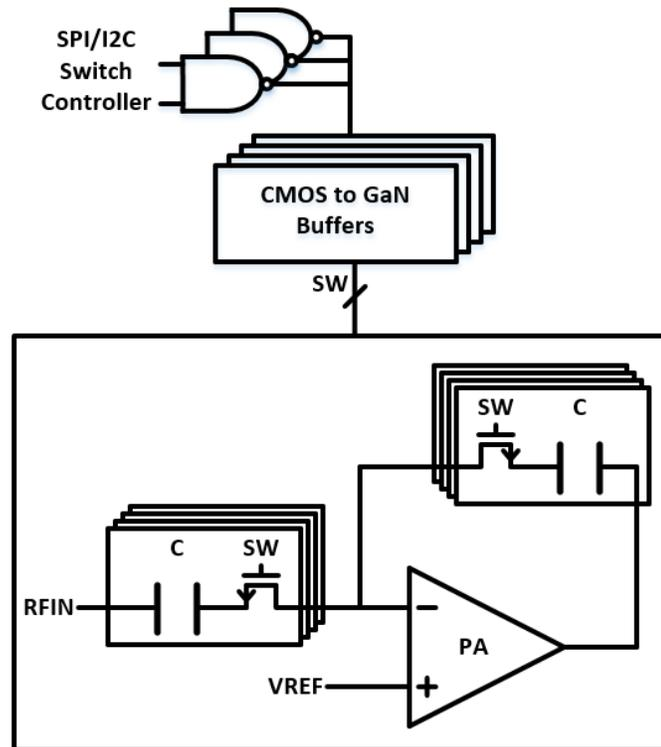
Figure 1.2: Demonstration of Variable Gain Control Requiring GaN Drivers
