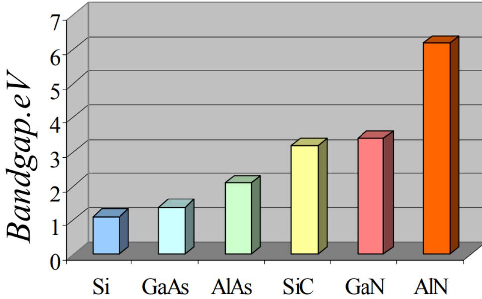
Figure 1.1: Bandgap of Semiconductor Materials [7]
