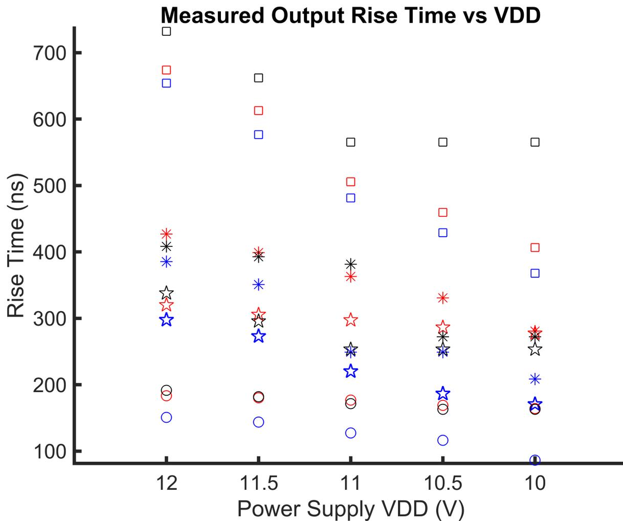
Figure A.3: Measured Output Rise Time
