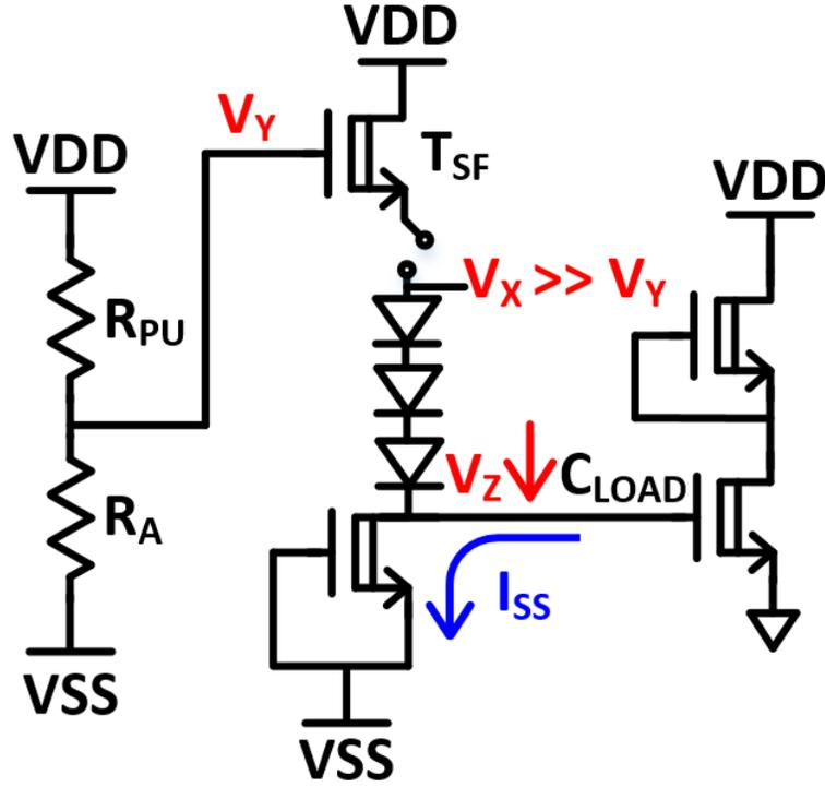
Figure 4.4: BFL INV Gate with Resistor Divider at Gate of  $T_{SF}$
