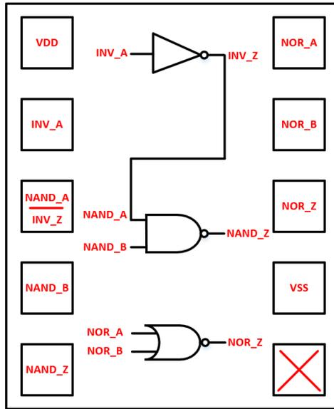
Figure 5.2: Gate Structure of A1/A3 Logic Banks
