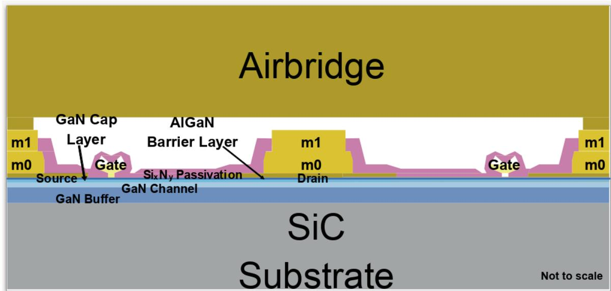
Figure 2.1: GaN Process pHEMT Topology
