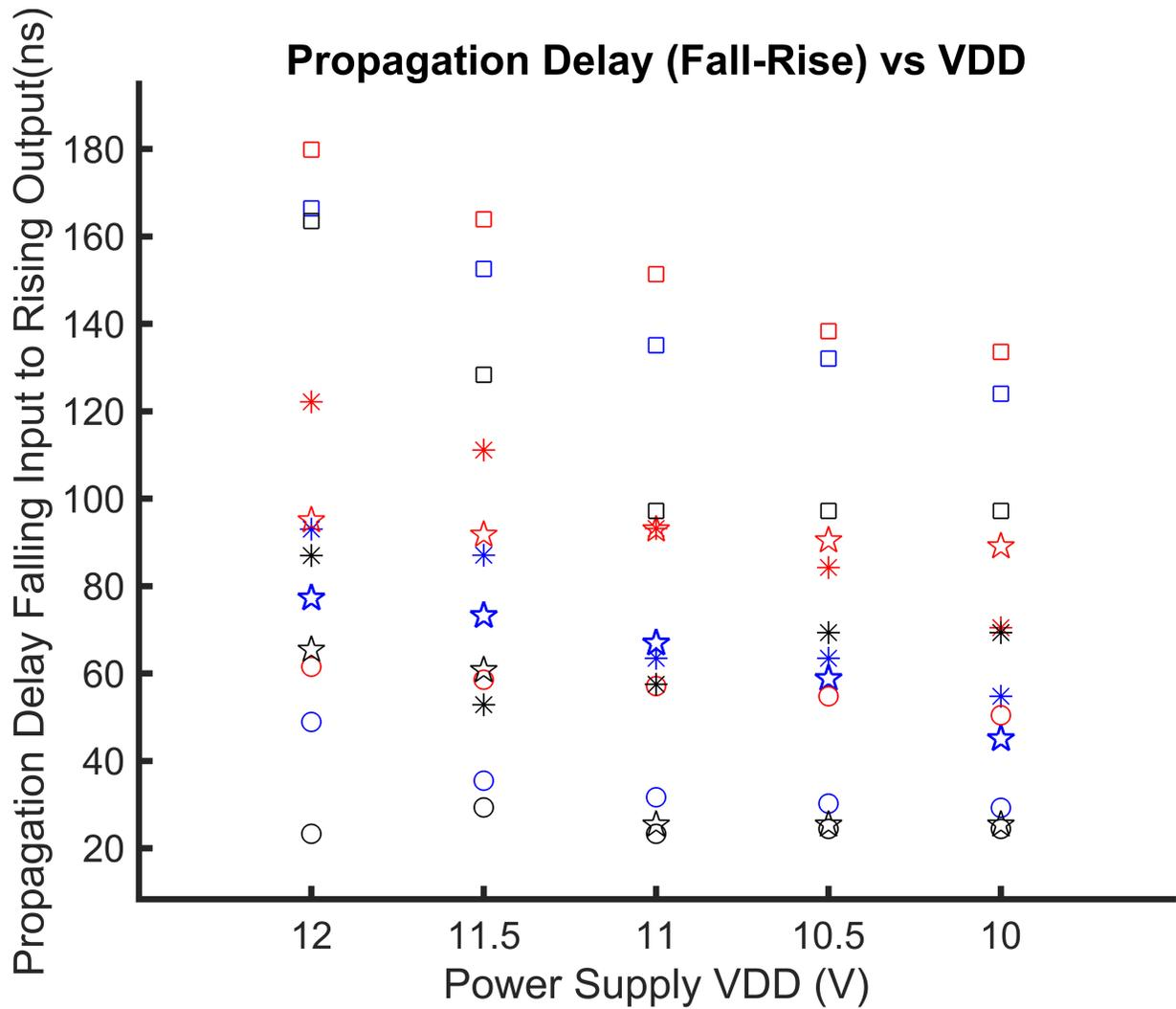
Figure A.8: Input Fall to Output Rise Propagation Delay
