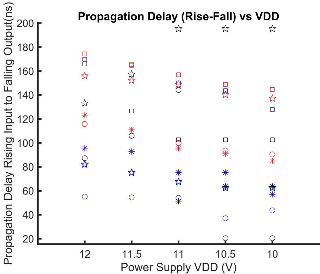
Figure A.9: Input Rise to Output Fall Propagation Delay
