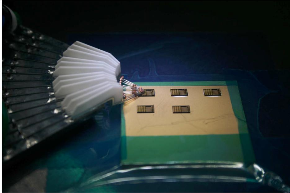
Figure 5.4: 10 Pin Probe Interfacing with GaN Logic Gates
