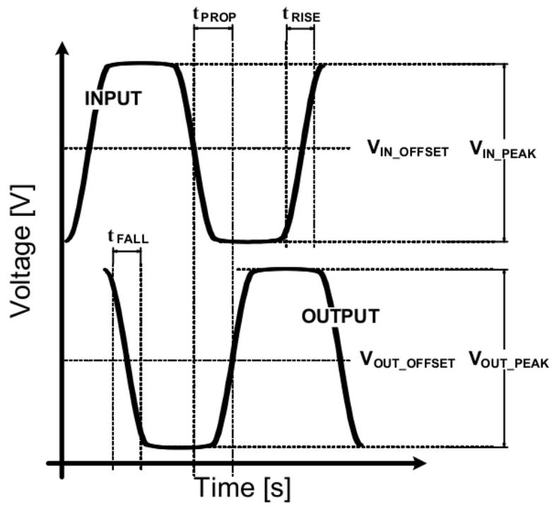
Figure 5.5: Digital Logic Performance Metrics for Gate Level Devices
