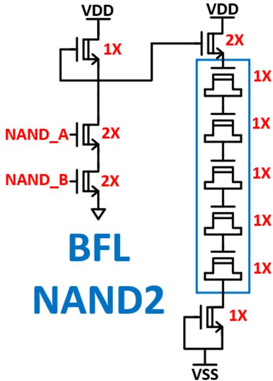
Figure 4.7: BFL NAND2 with Diode Connected Level Shifting
