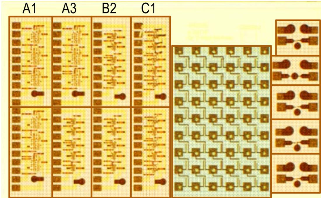
Figure 5.1: Designed Logic Gates on Gold-Plated Copper Tungsten Carrier
