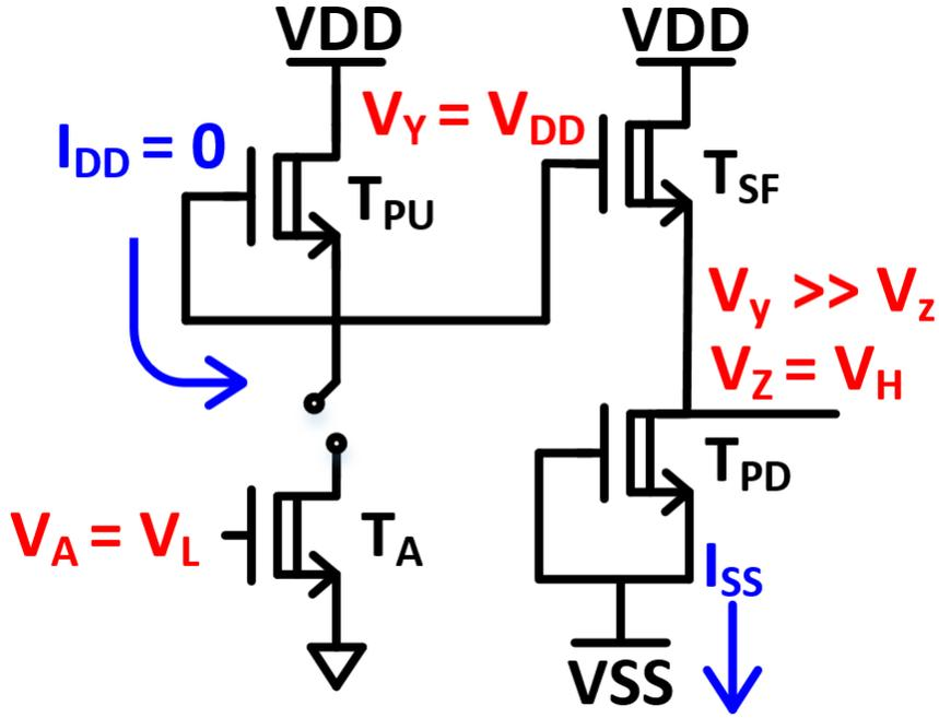
Figure 4.1: BFL INV Gate without Level Shifting Diodes
