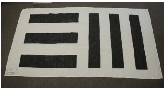
Fig. 8—NIIRS 5 (left) and NIIRS 6 to 9 (right) optical bar target for imagery quality measurement
