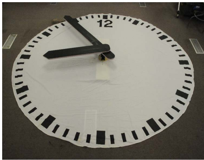
Fig. 7—3 m diameter analog clock for time-on-target tracking
