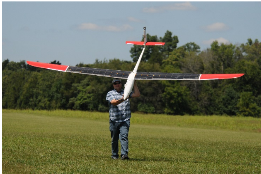
Fig. 3—NRL's PV-SBXC UAV used for flight experiments
