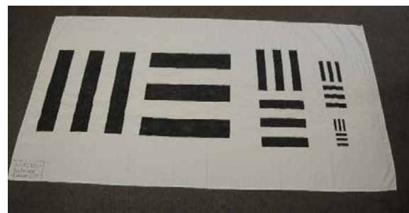
Fig. 8—NIIRS 5 (left) and NIIRS 6 to 9 (right) optical bar target for imagery quality measurement
