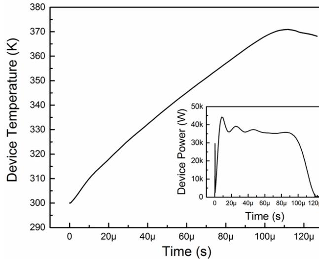
**Fig. 7** Simulated temperature and dissipated power of SiC SGTO with a 120- $\mu$ s pulse at 2 kA
