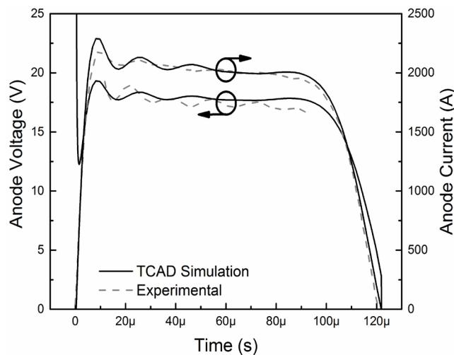
**Fig. 6** Experimental and simulated (non-isothermal) 15-kV SiC SGTO anode voltage and current waveforms during a 120- $\mu$ s 2-kA PFN switching cycle; the concordance between the experimental and simulated waveforms demonstrates the accuracy of the TCAD model
