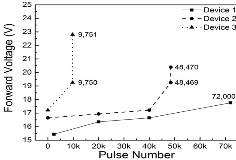
**Fig. 8** Experimental  $V_F$  measured throughout the 2-kA, 120- $\mu$ s pulsed evaluation of SiC GTOs until failure
