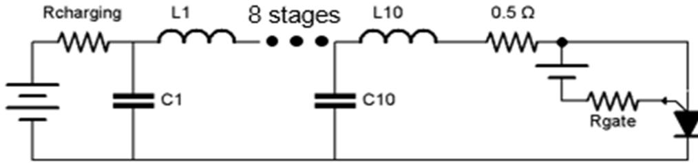
**Fig. 2** MixedMode 10-stage PFN schematic for evaluating the pulsed characteristics of the SiC SGTO
