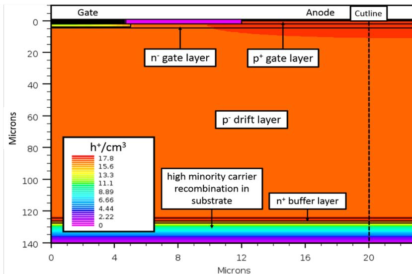
**Fig. 9** Simulated hole concentration profile throughout the device structure at a narrow current pulse of 2 kA revealing the exposure of high minority carrier injection into the substrate
