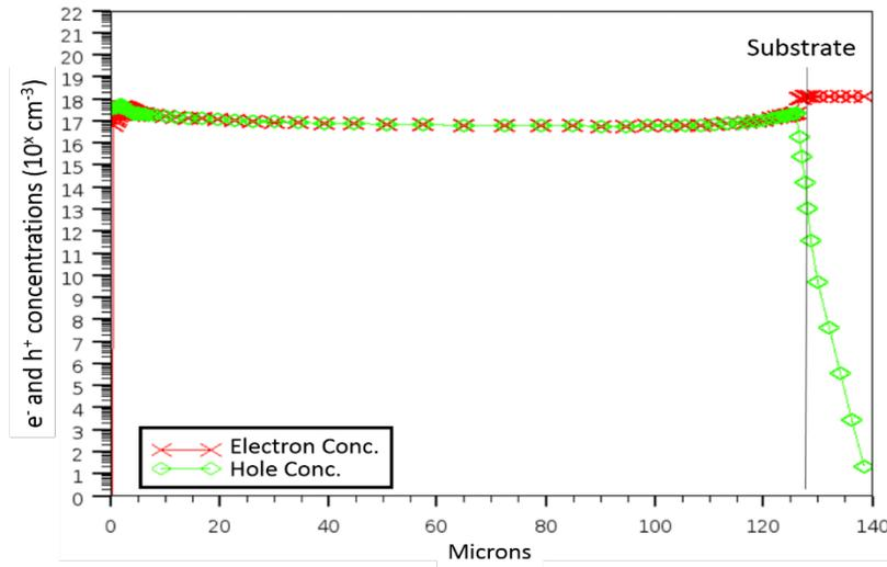
**Fig. 10** Simulated electron and hole concentrations along the y-axis cutline that further demonstrates the high ( $\sim 10^{14} \text{ cm}^{-3}$ ) minority carrier density injected into the substrate
