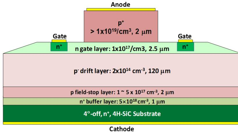
Fig. 1. Simplified schematic cross section of the 15-kV SiC SGTO (diagram not to scale)
