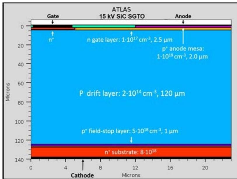
Fig. 4 SiC SGTO half unit cell as simulated in Silvaco Atlas
