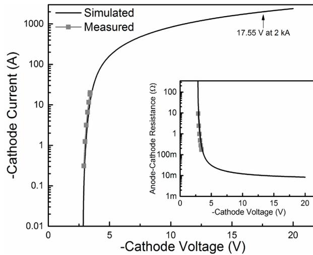
**Fig. 5** Experimental and simulated (isothermal) 15-kV SiC SGTO forward characteristics displaying strong similarity
