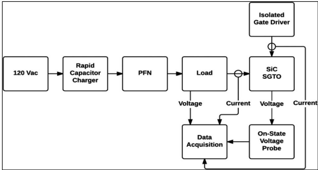
Fig. 3 Simplified block diagram of the pulse evaluation system to characterize high-voltage SiC SGTO
