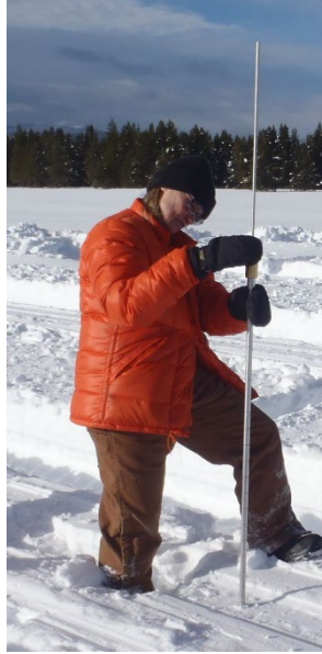
Figure 4. CRREL's Dr. Sally Shoop using the ram to measure the hardness of a vehicle belly drag after a coast-down test at NATC.
