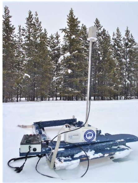
Figure 2. The SMP mounted on a sled at the West Yellowstone airfield during the NATC campaign. The SMP was developed and designed by Dr. Martin Schneebeli (SLF) and Dr. Jerome Johnson (CRREL) in the mid-1990s. The pictured sled was designed and built by Dr. Matthew Sturm (CRREL).
