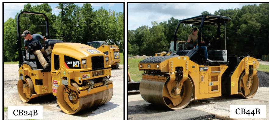
Figure 2.10. Steel wheel roller compactors.
