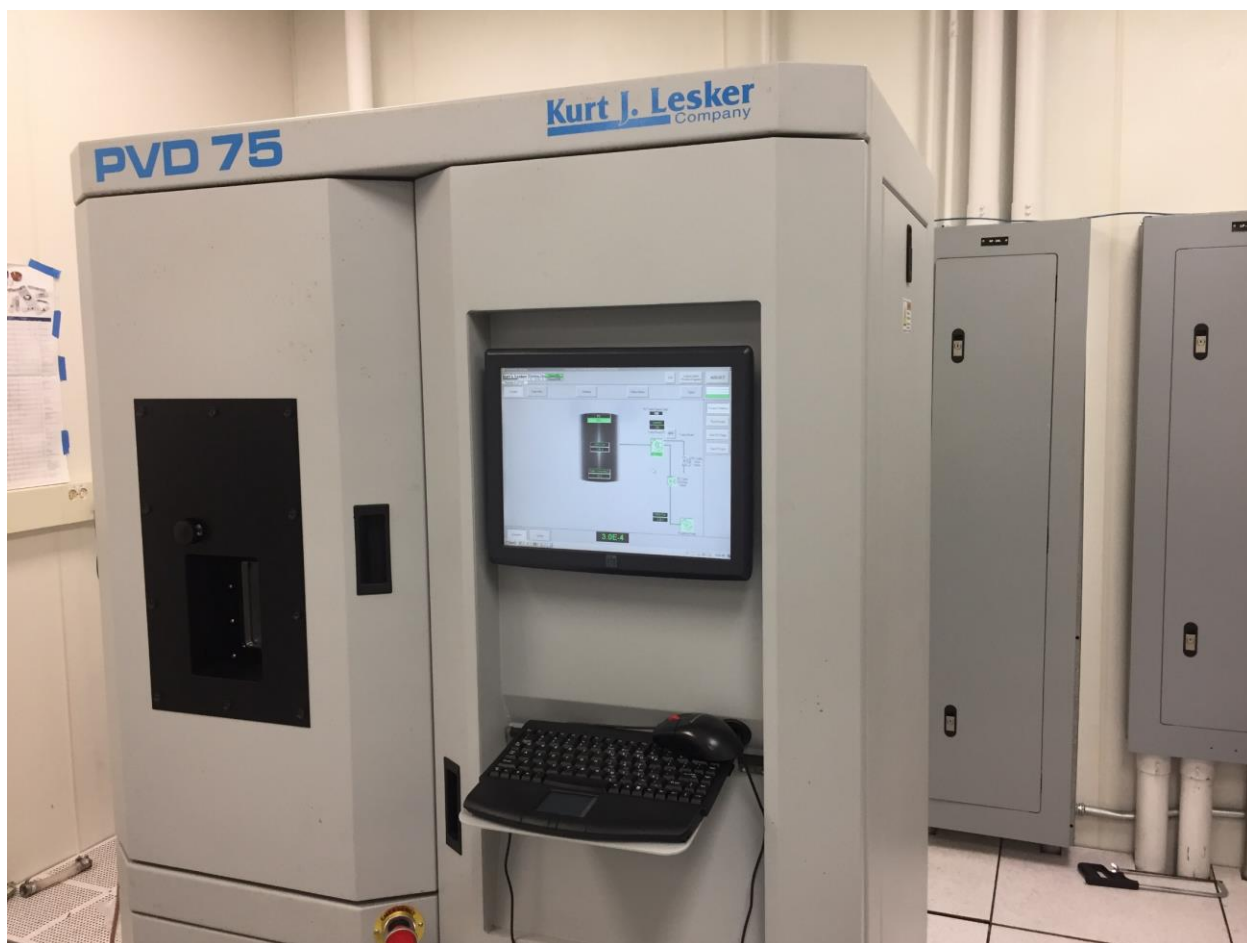
Figure 6. The upgraded e-beam evaporation system with a new four-pocket e-beam source.
