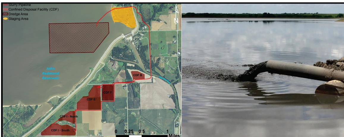
Figure 2. John Redmond Reservoir dredging diagram (left); dredging discharge into CDF E (right).
