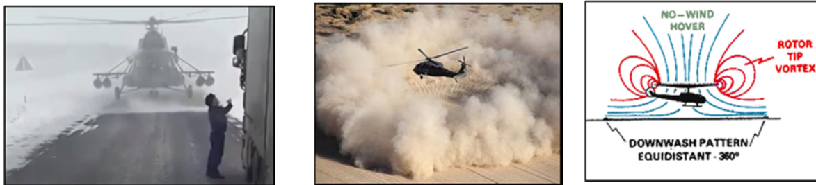
Figure 4. Examples of rotor downdraft. The rotor downdraft, in combination with the rotor tip vortex, creates an effect that scatters loose ground material (sand and/or snow, in the cases shown) [from the Army Combat Photographer collection].
