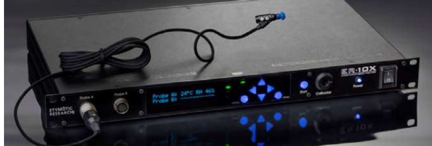
Figure 7. Etymotic ER-10X Extended bandwidth probe system.
