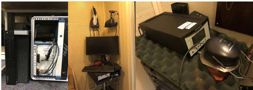
Figure 3. Station 1 equipment. Left: Control PC, NI PXI system, and ViAcoustics response box. Center: remote PC monitor, Titan system (upper left), video otoscope (upper right). Right: Sennheiser HD 200 headphones, Brüel & Kjær Nexus microphone power supply, and artificial ear.
